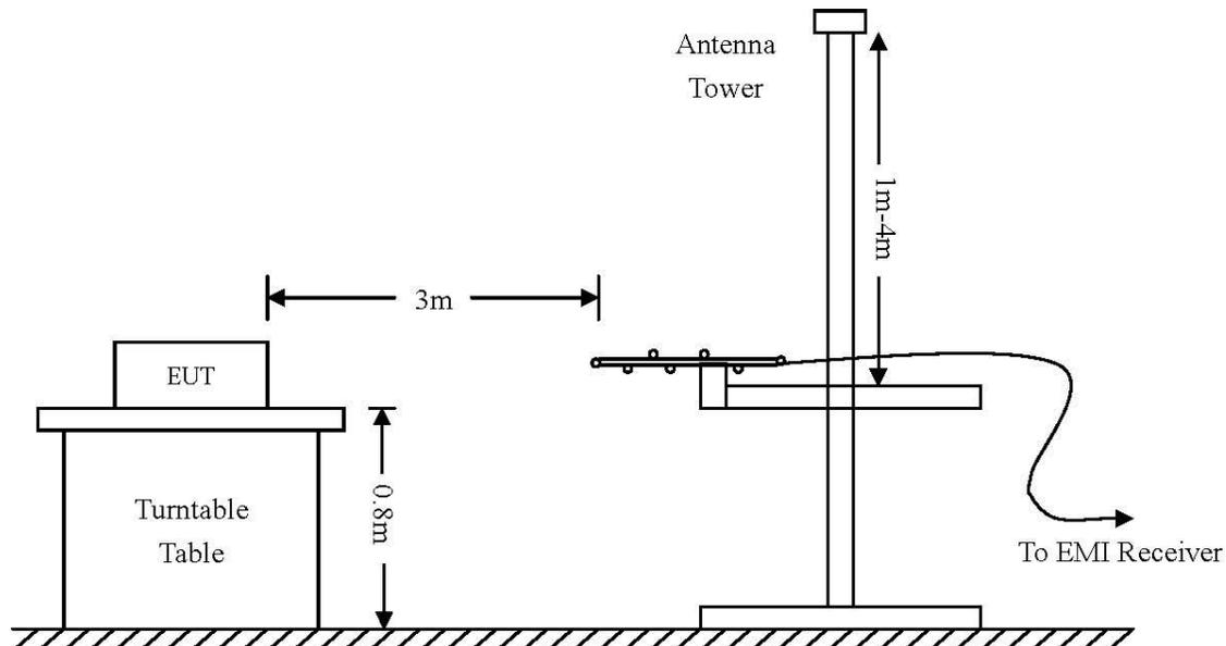
**Diagram 1 Test arrangement for radiated emissions tested on Open Area Test Site (OATS)**
