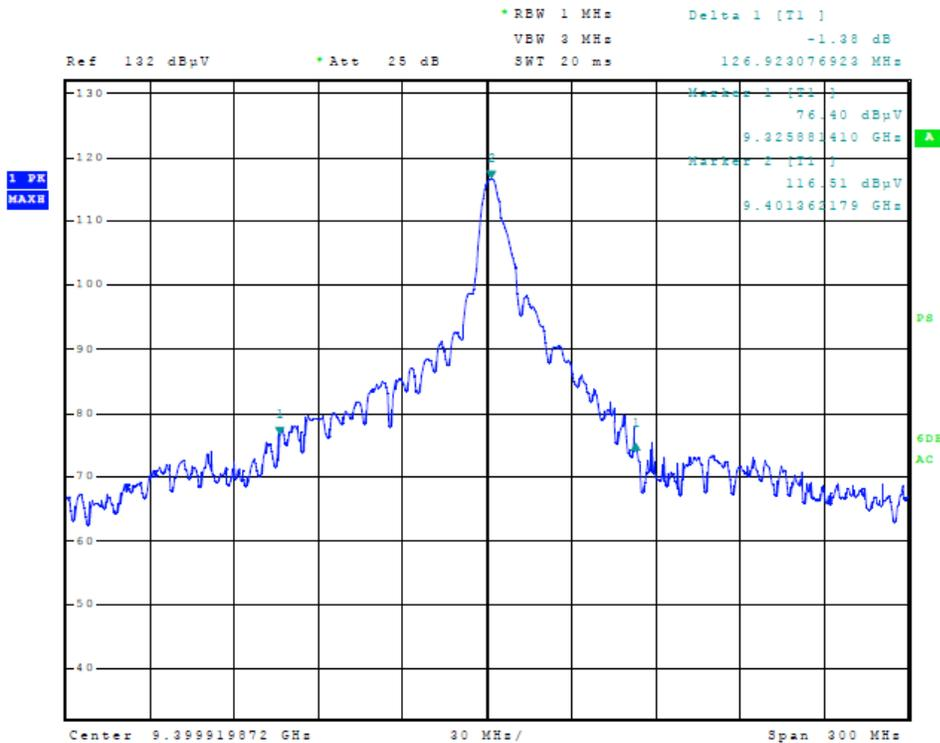
Figure 3 Plot of analyzer screen showing 40-dB occupied bandwidth (1/2 nm)
