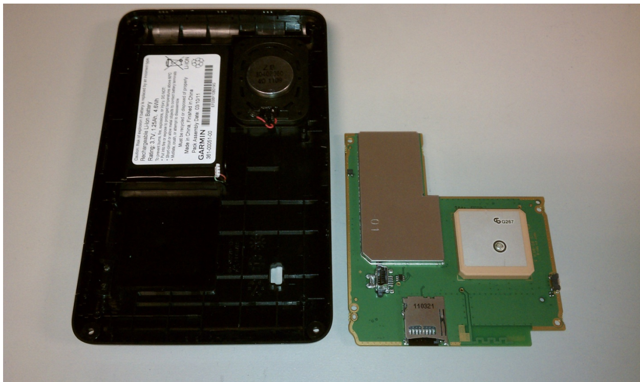
Inside Rear Case and PCB
