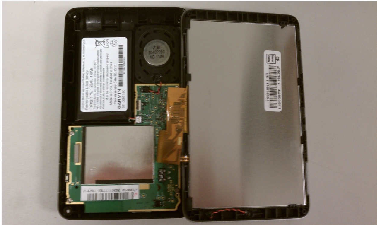
Inside Rear Case and PCB
