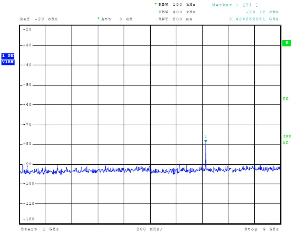
**Figure Twenty-Three Receiver Temporary Antenna Port Conducted Emissions**
