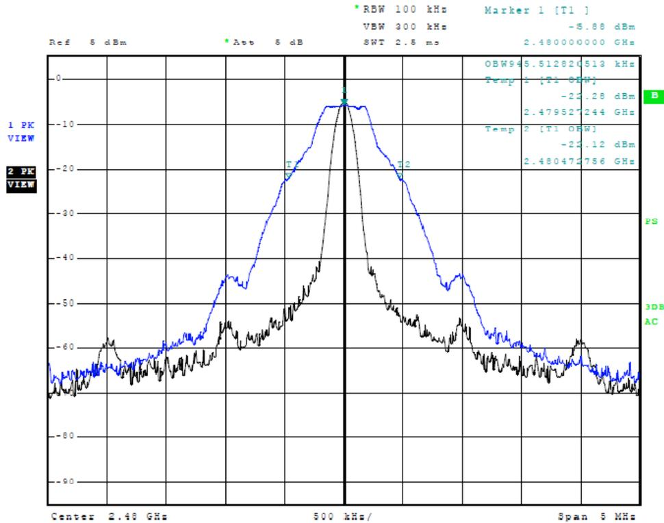
Figure Twelve Plot of Occupied Bandwidth (High channel)
