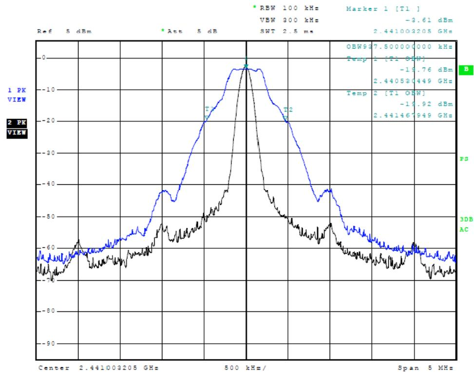
Figure Eleven Plot of Occupied Bandwidth (Middle channel)
