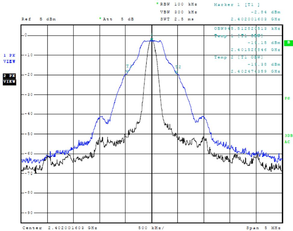
Figure Ten Plot of Occupied Bandwidth (Low channel)
