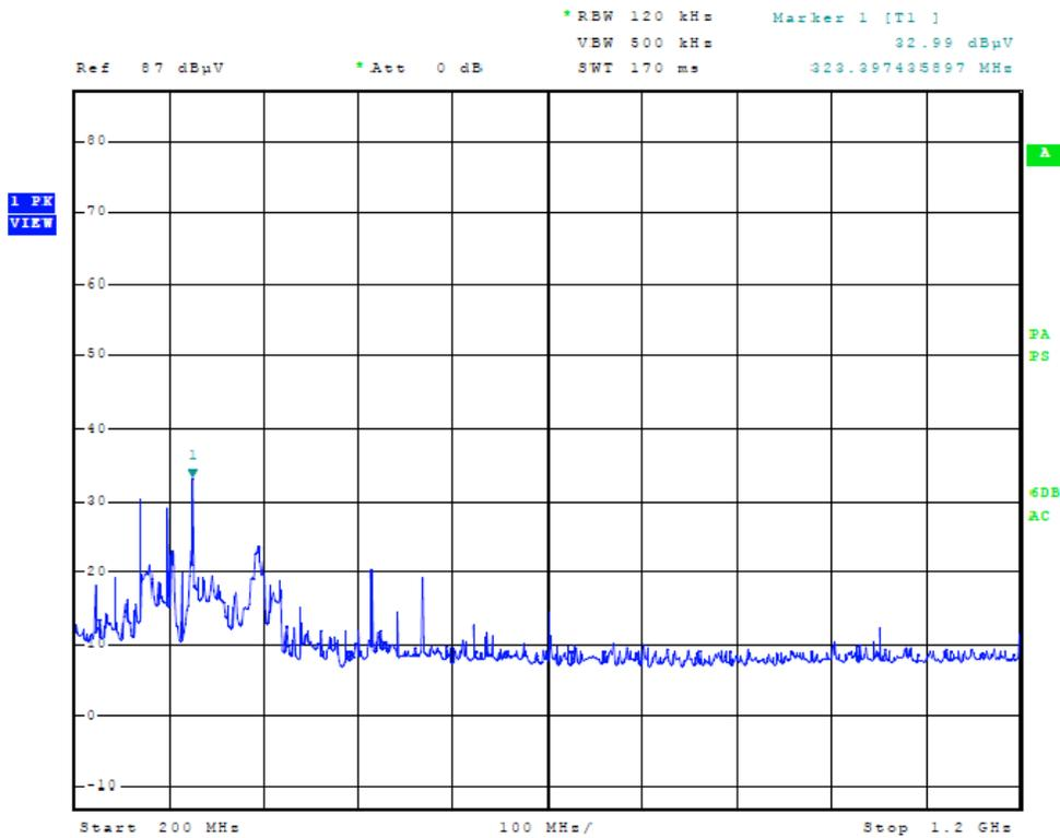
**Figure Four Plot of General Radiated Emissions (EUT CLA)**
