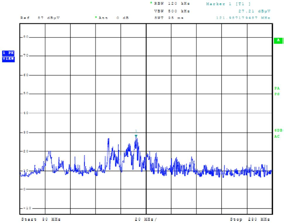
**Figure Three Plot of General Radiated Emissions (EUT CLA)**
