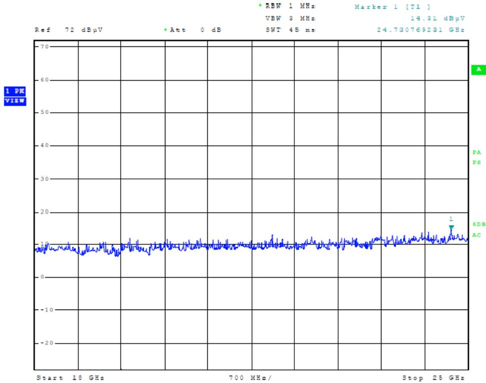
**Figure Eleven Plot of General Radiated Emissions**
