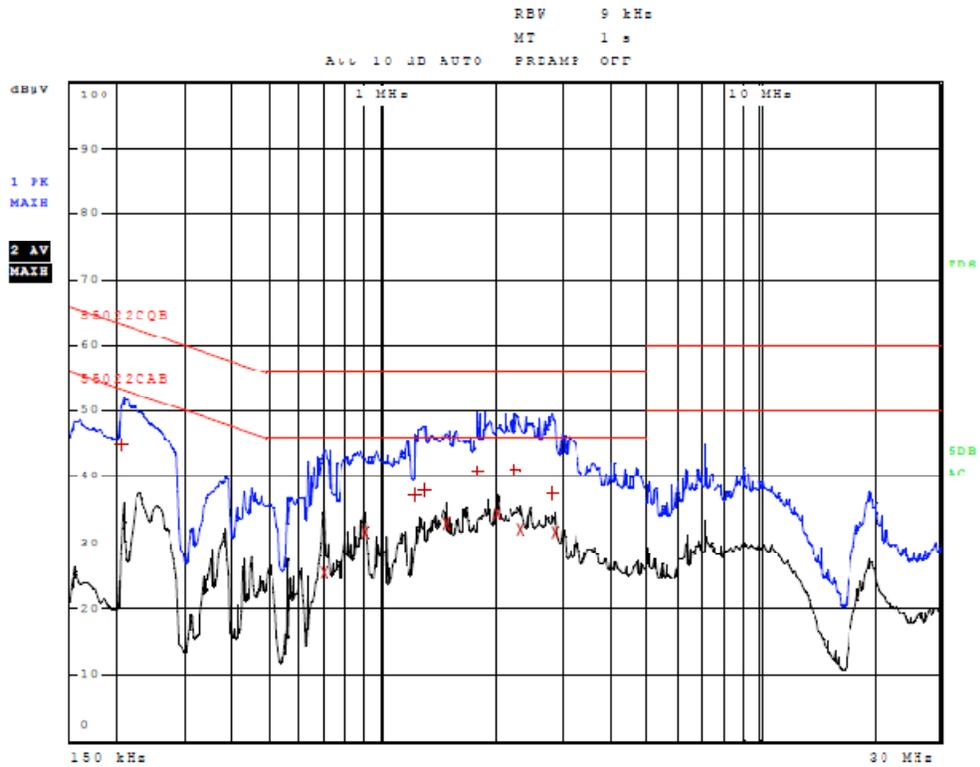
Figure Four AC Line Conducted emissions of EUT line 2 (EUT USB CPU)
