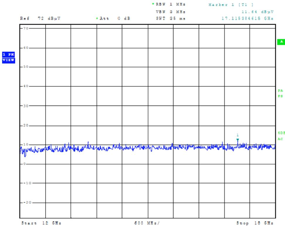
Figure Ten Plot of General Radiated Emissions
