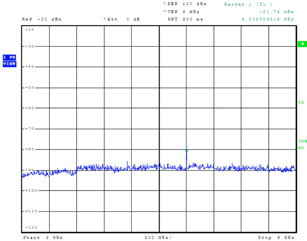
**Figure Twenty-two Receiver Temporary Antenna Port Conducted Emissions**
