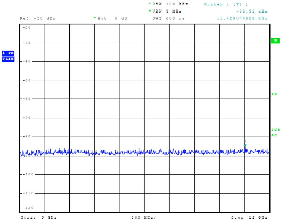
**Figure Twenty-one Receiver Temporary Antenna Port Conducted Emissions**
