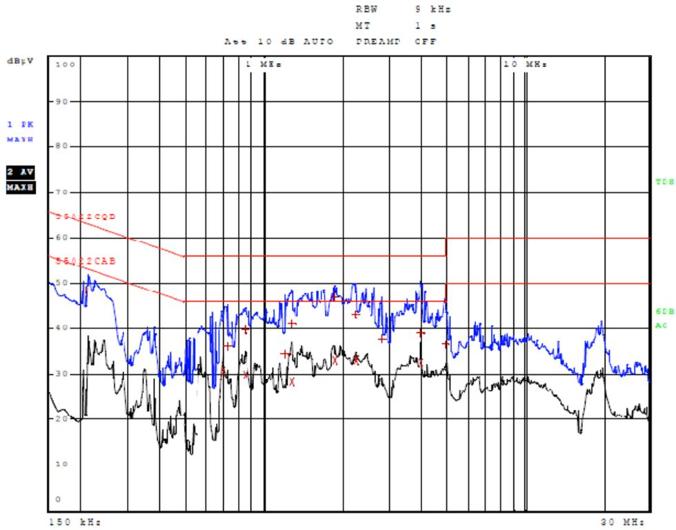
Figure Three AC Line Conducted emissions of EUT line 1 (EUT USB CPU)
