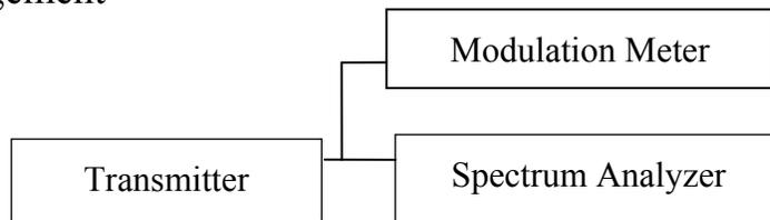
The radio frequency output would be coupled to Spectrum Analyzer and modulation meter. The spectrum analyzer would be used to observe the radio frequency spectrum with the transmitter operating in its various modes. The modulation meter would be used to measure the percent modulation or frequency deviation.
