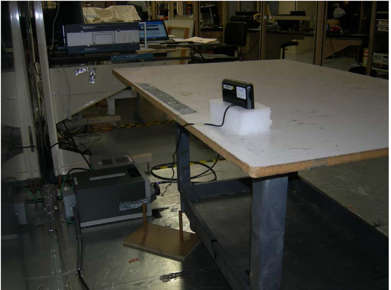
**Figure 3: Conducted Emissions – Wall Charger**
