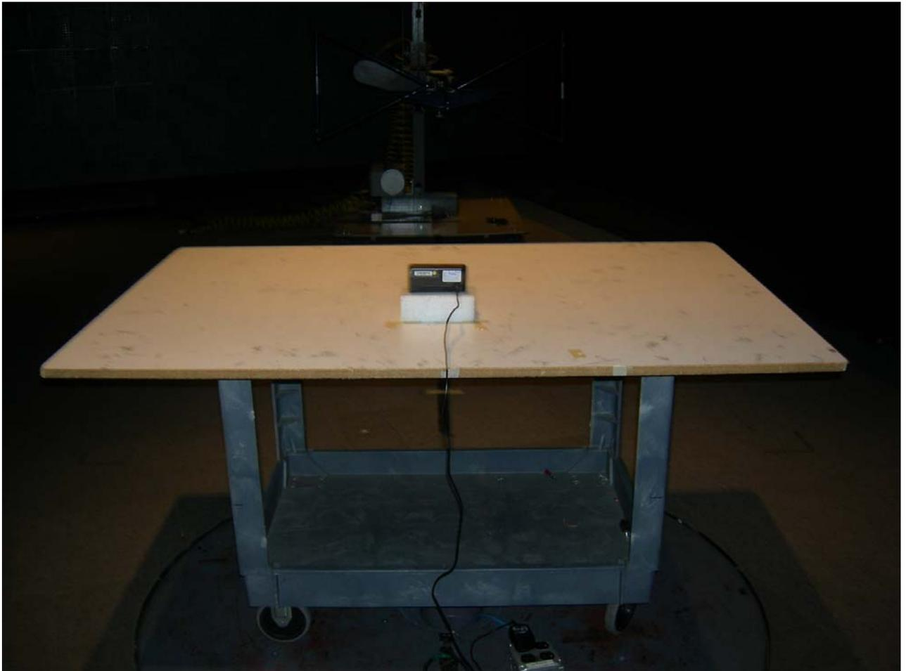
**Figure 8: Radiated Emissions – Unintentional – Wall Charger**
