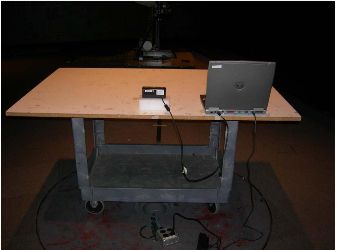
**Figure 10: Radiated Emissions – Unintentional – PC Charger**
