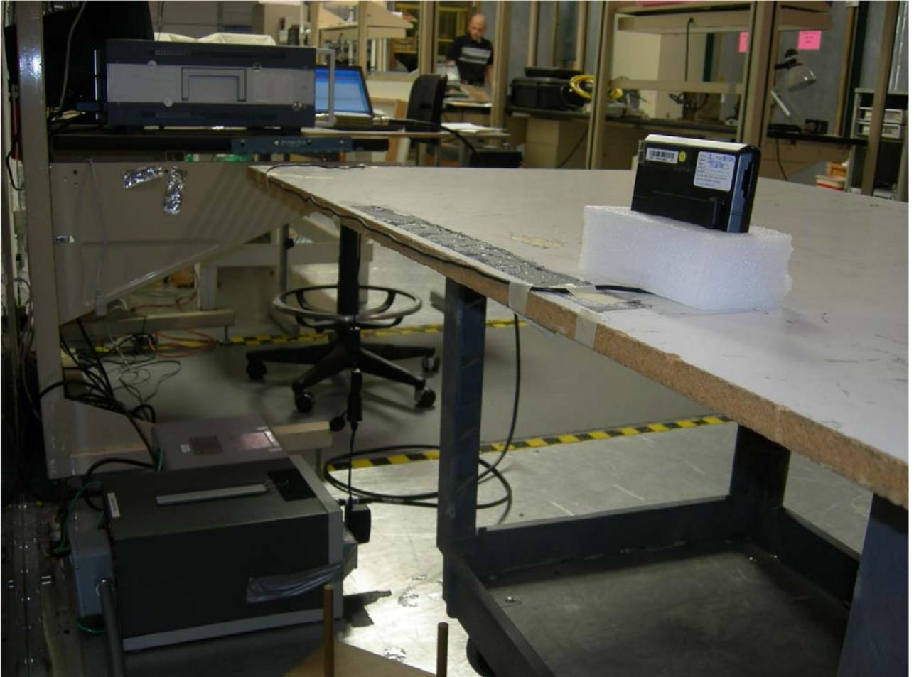
**Figure 4: Conducted Emissions – Car Charger**
