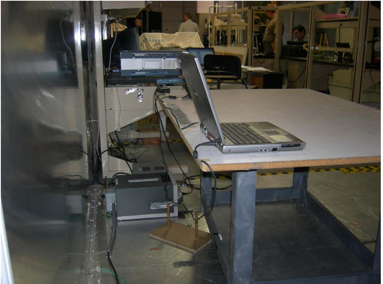
**Figure 6: Conducted Emissions – PC Charger**
