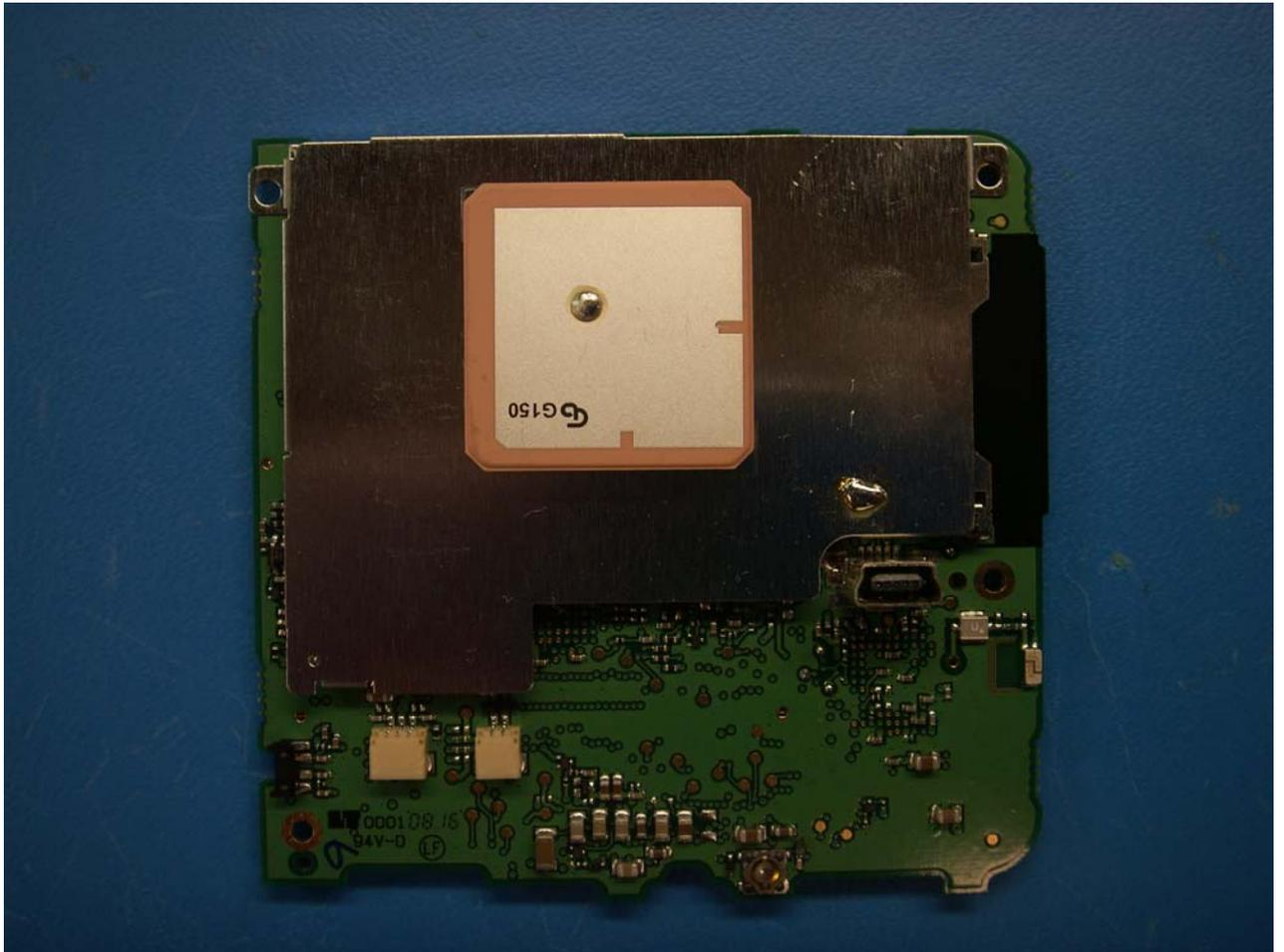
**Figure 3: Bottom View with Shields**
