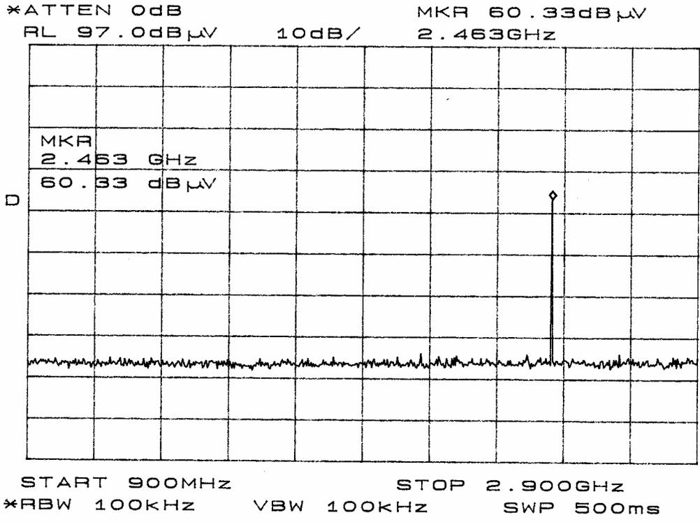
Figure eleven Radiated Emissions Plot
