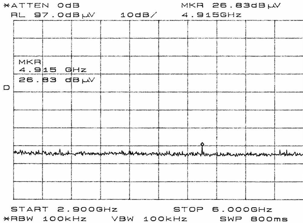
Figure twelve Radiated Emissions Plot
