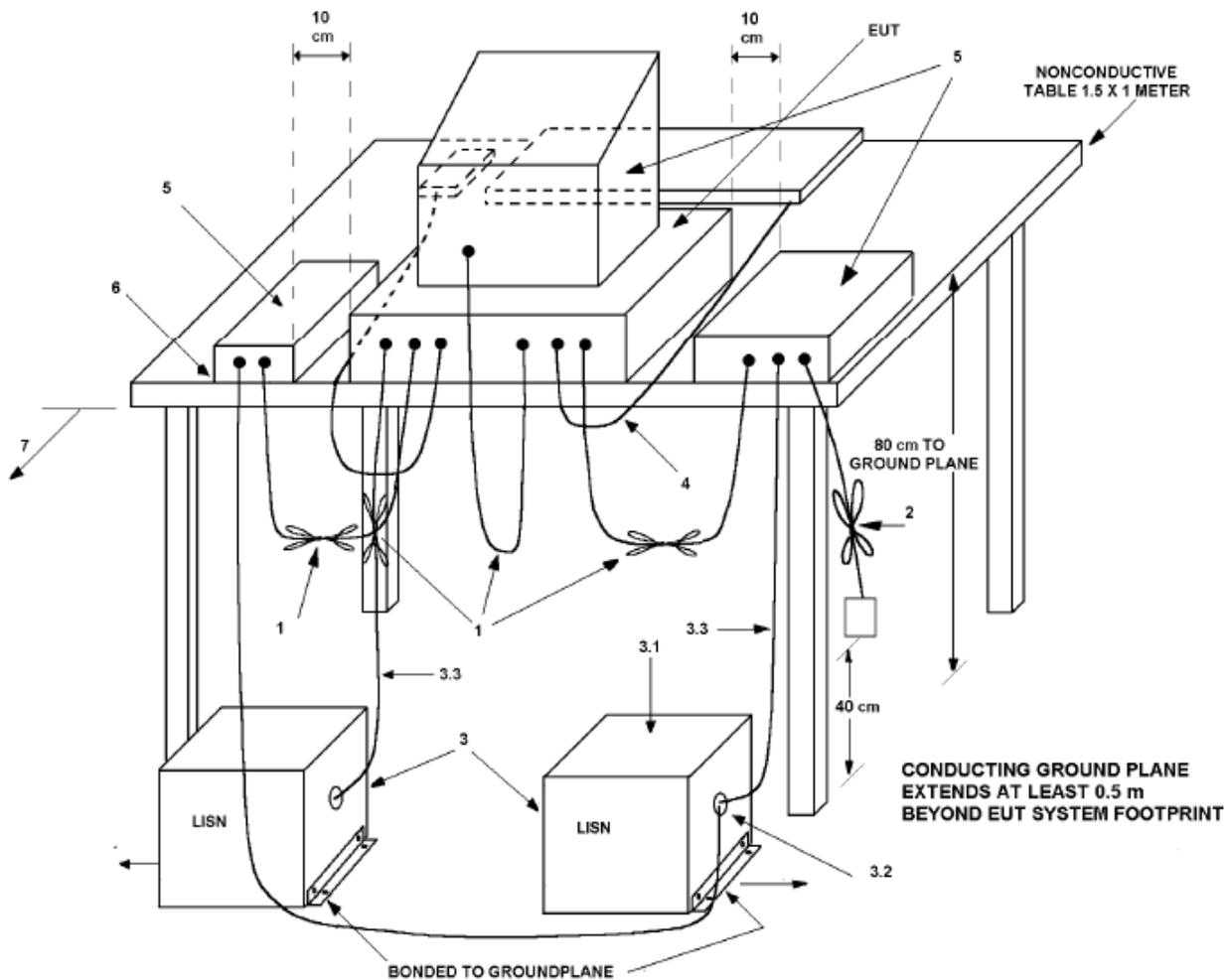
1. Interconnecting cables that hang closer than 40 cm to the ground plane were folded back and forth in the center forming a bundle 30 cm to 40 cm long.
