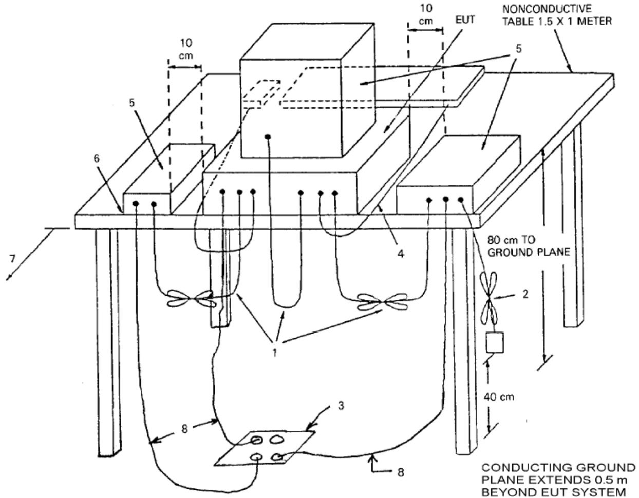
1. Interconnecting cables that hang closer than 40 cm to the ground plane shall be folded back and forth in the center, forming a bundle 30 cm to 40 cm long.
