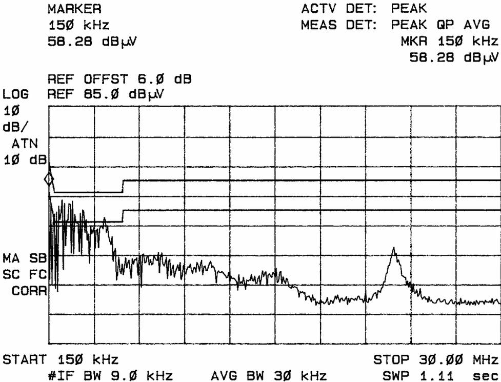
Figure two Conducted emissions of EUT line 2
