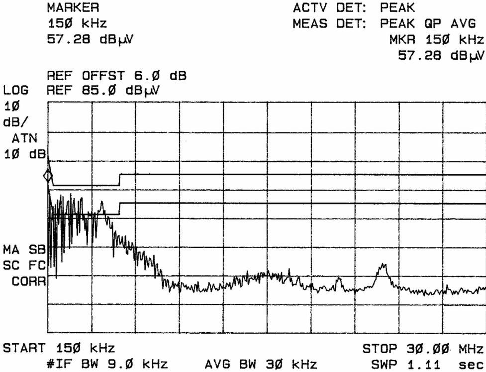
Figure one Conducted emissions of EUT line 1
