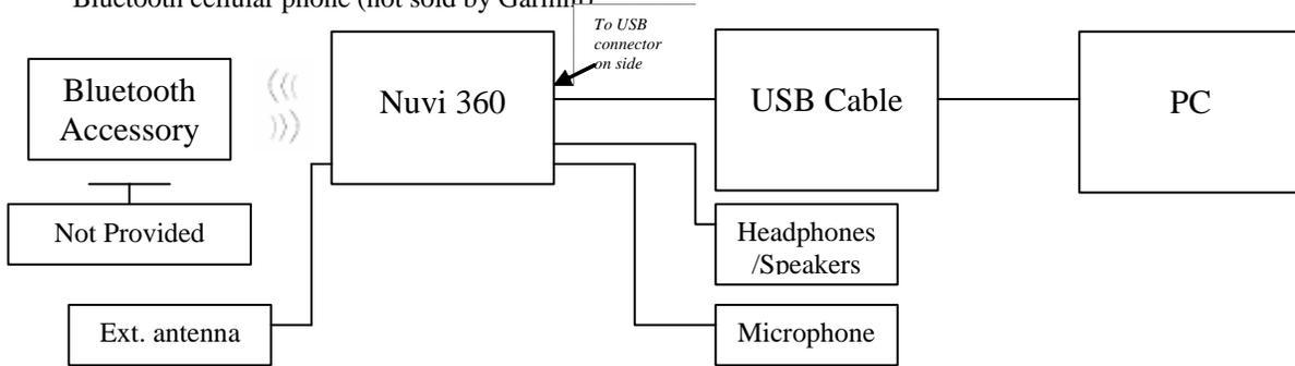
2. nuvi 360 connected to GTM 10 TMC FM traffic receiver (GPN: 011-01150-0x). Powered by cigarette lighter adapter (GPN: 320-00239-21). 2.5mm and 3.5mm jacks available for audio input/output. Can be used with external antenna (GPN: 011-00149-05). Can be connected to a Bluetooth wireless accessory e.g. Bluetooth cellular phone (not sold by Garmin).
