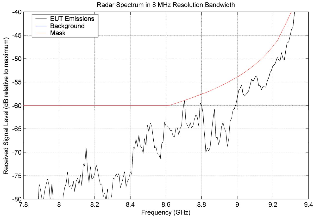
Figure 6. Emission measurement data detail from 7.8 to 9.4 GHz.
