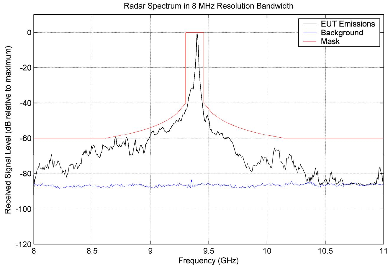
Figure 4. Center frequency portion of the spectrum.
