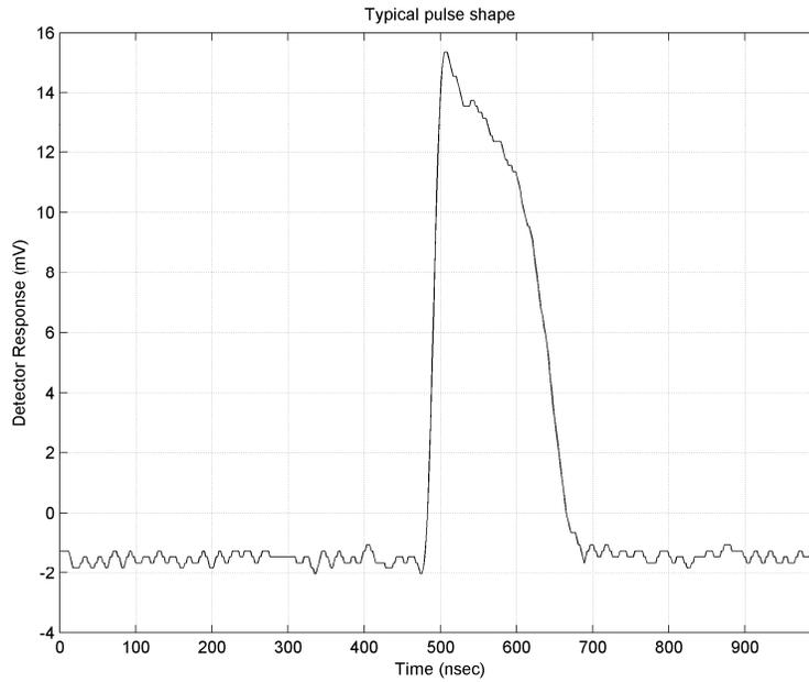
Figure 2. Typical pulse from EUT using wideband detector.
