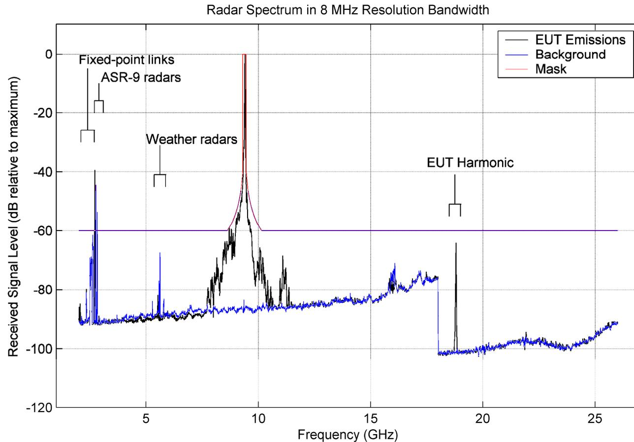
Figure 3. EUT Emissions 2 – 26 GHz.
