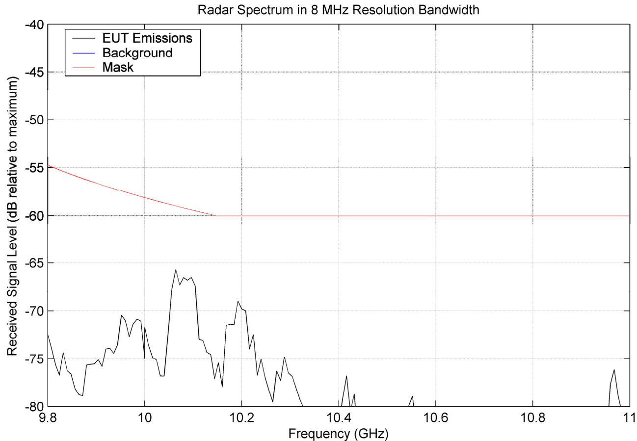
Figure 7. Emission measurement data detail from 9.8 to 11 GHz.
