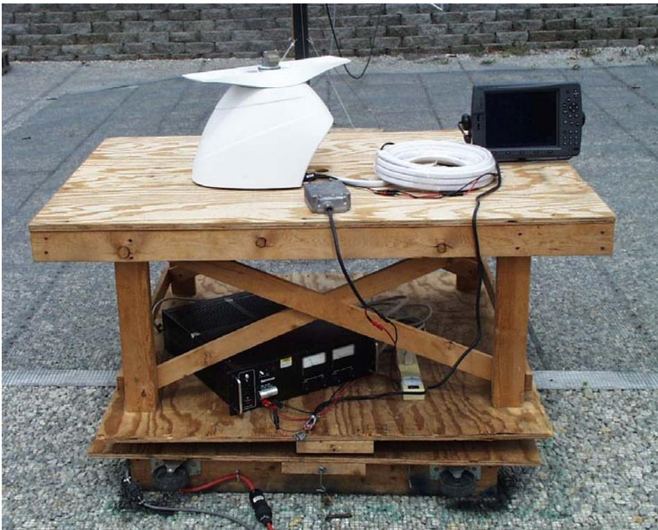
10-meter test setup with 4-foot antenna connected.
