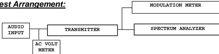
The radio frequency output was coupled to a HP Spectrum Analyzer and a modulation meter. The spectrum analyzer was used to observe the radio frequency spectrum with the transmitter operating in its various modes. The modulation meter was used to measure the percent modulation or frequency deviation.
