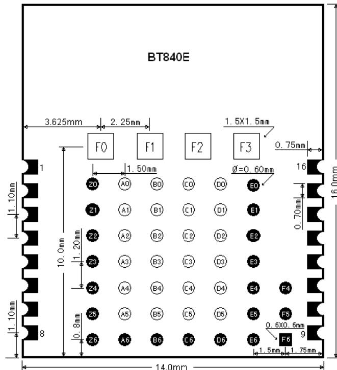
BT840N and BT840NE mechanical drawings, top view.
