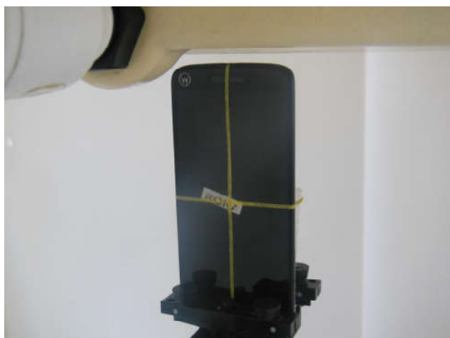
Bottom Side, Test Separation 5 mm
