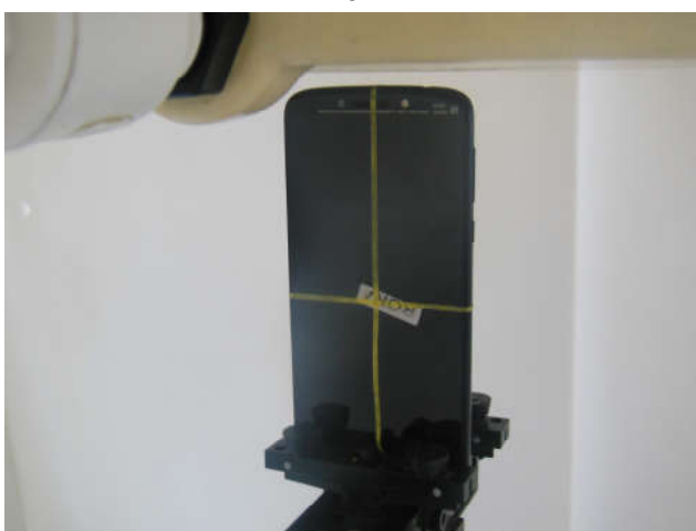
Top Side, Test Separation 5 mm
