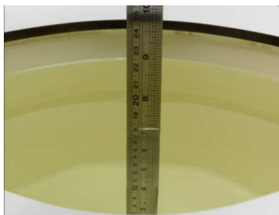
Fig 10.2 Photo of Liquid Height for Body SAR
