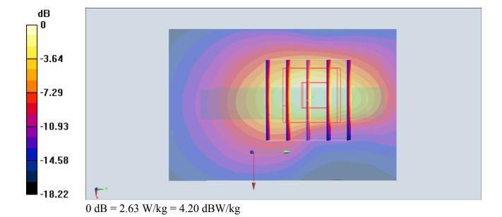
Communication System: WCDMA; Frequency: 1752.6 MHz; Duty Cycle: 1:1
