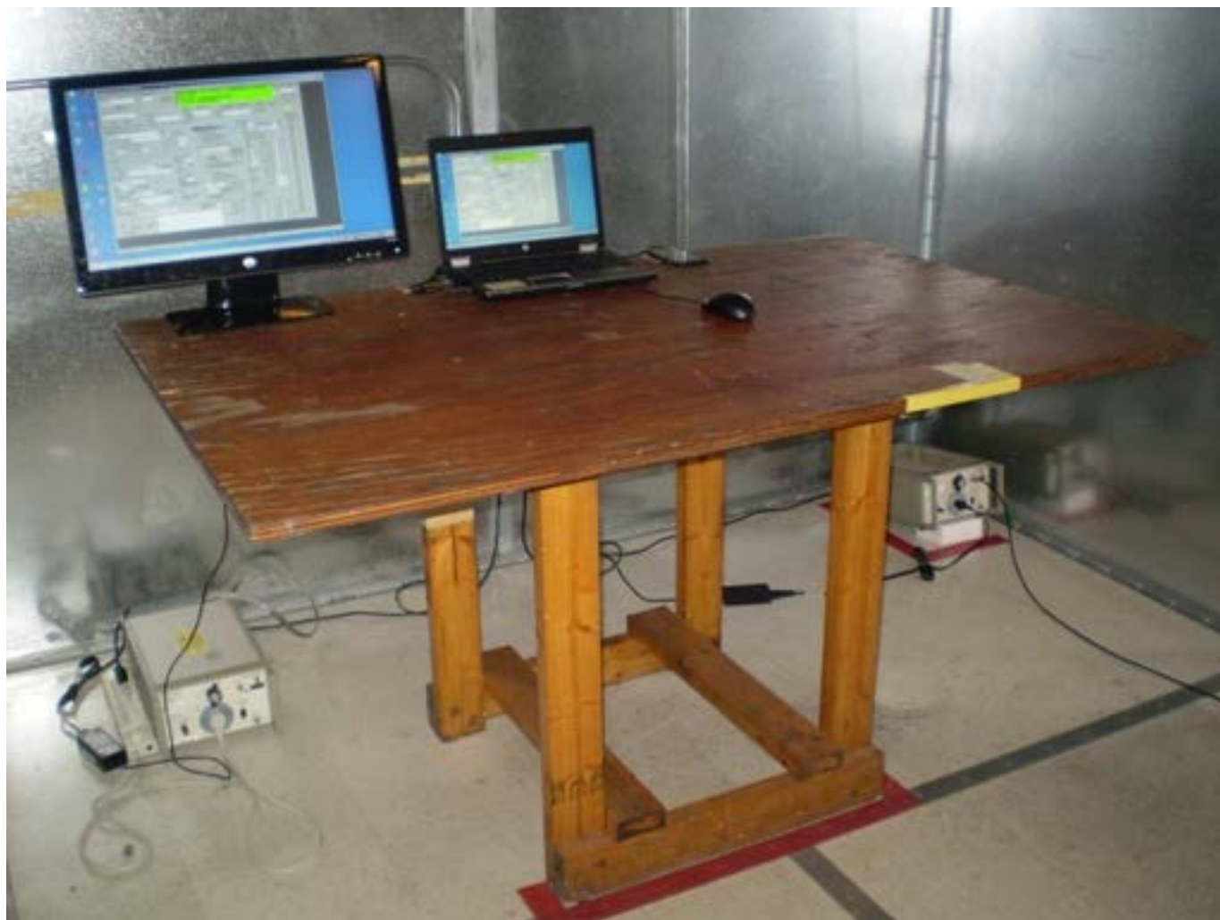
Figure 7c3-1: Test Configuration – AC Line (Part 15 Computing Device).
