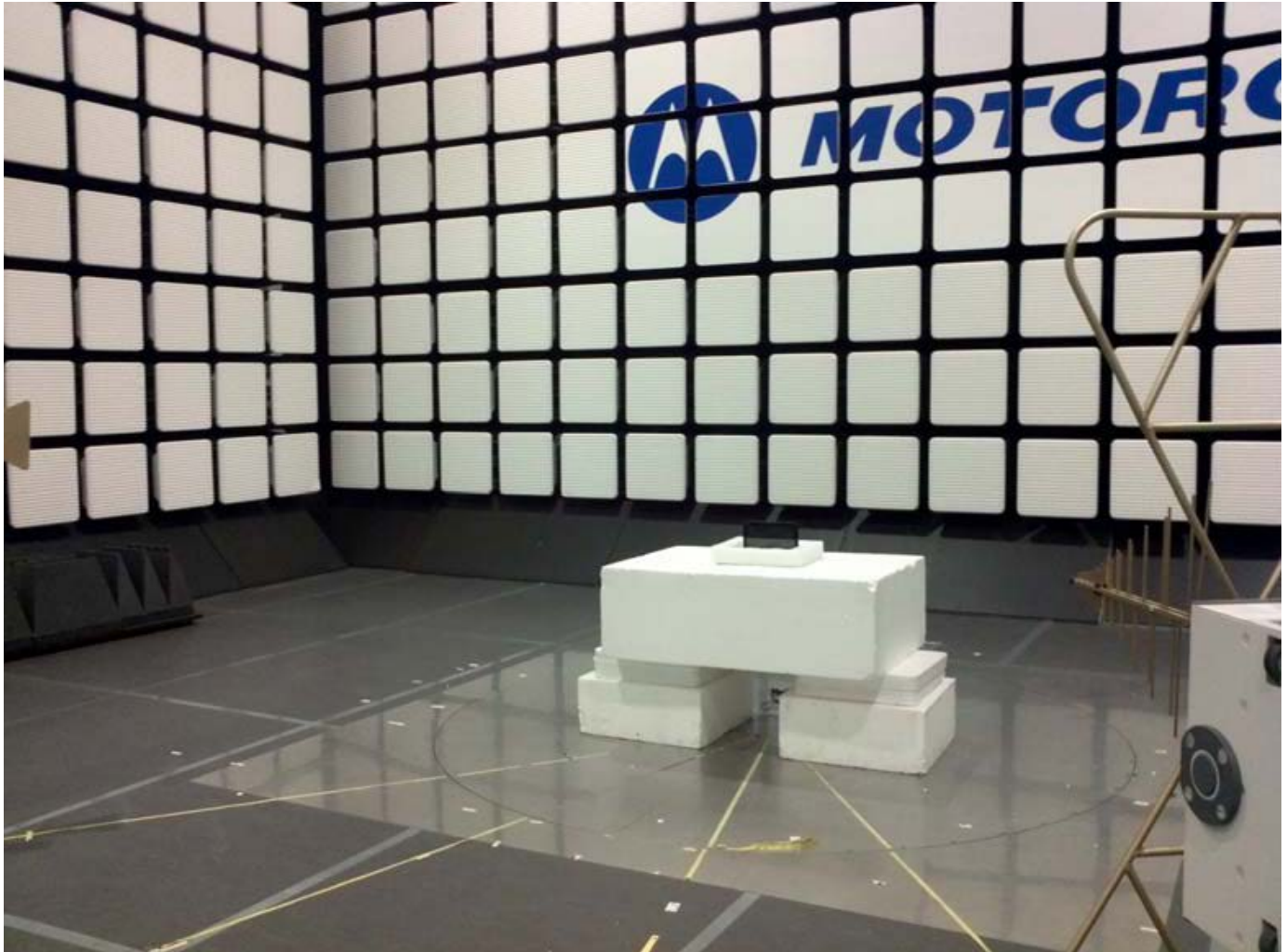
Figure 7c1-1: TX Radiated Emissions Configuration.
