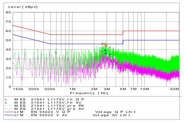
1900 EV-DO Rev0 FTAP Channel 1175 - Tx Mode - Line Coupling
