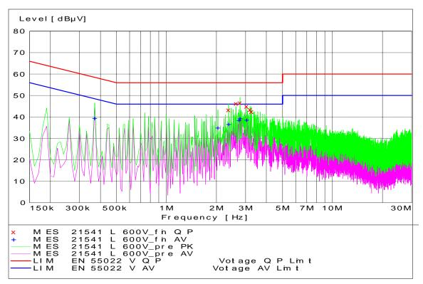
1900 EV-DO Rev0 FTAP Channel 600 - Tx Mode - Line Coupling
