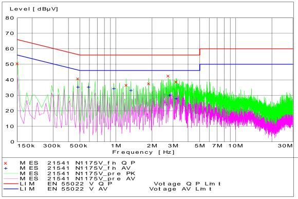
1900 EV-DO Rev0 FTAP Channel 1175-Tx Mode-Neutral Coupling
