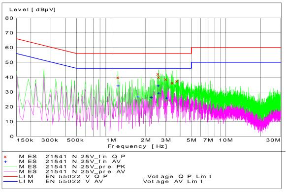
1900 EV-DO Rev0 FTAP Channel 25 - Tx Mode - Neutral Coupling
