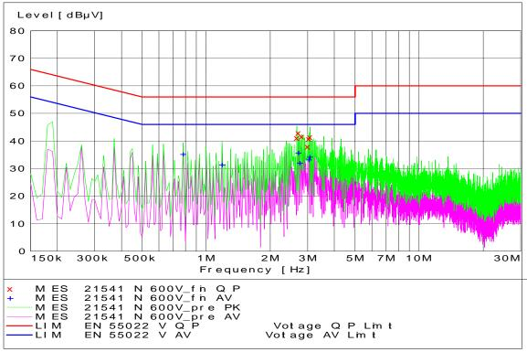
1900 EV-DO Rev0 FTAP Channel 600-Tx Mode - Neutral Coupling
