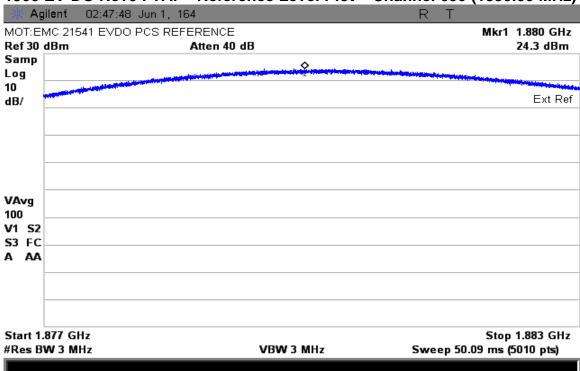
1900 EV-DO Rev0 FTAP-Occupied Bandwidth-Channel 600 (1880.00 MHz)
