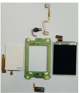
LCD Module & FLIP Rigid PCB & CLi & Hinge Flex PC & Vibrator & Ear Piece
