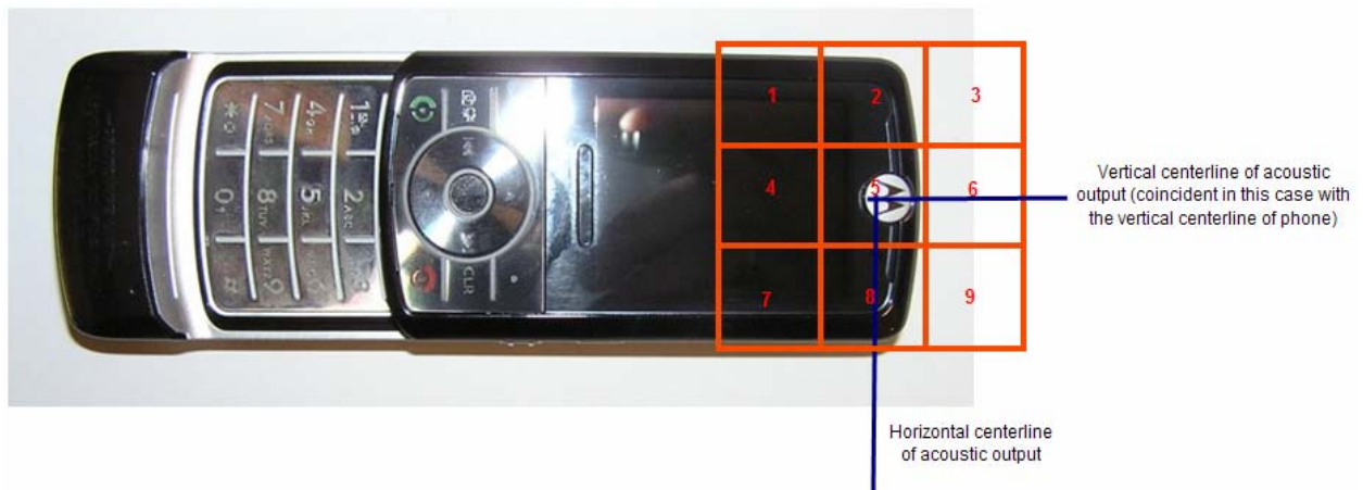
Figure A5-2. Phone Open - Orientation of Wireless Device and Measurement Plane
