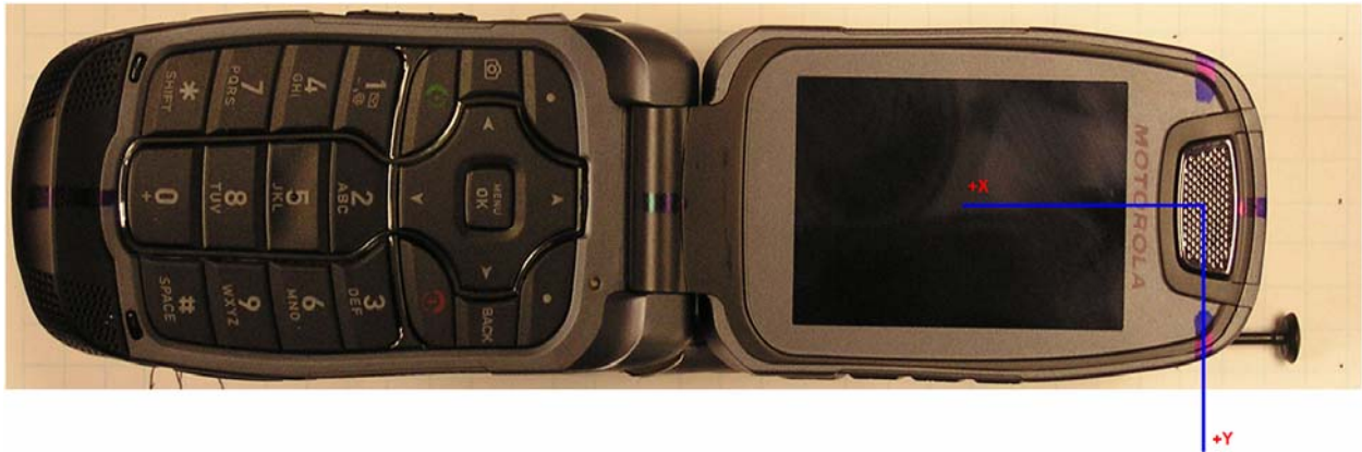
Figure A4-4. Phone Open – Coordinate Axis for T-coil Measurements
