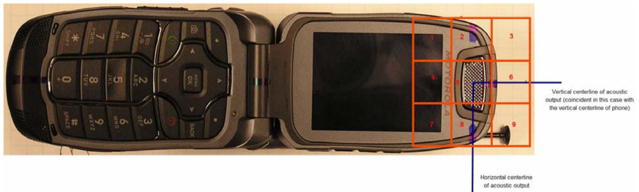
Figure A4-6. Phone Open – 5 cm x 5 cm grid for Near Field Measurements
