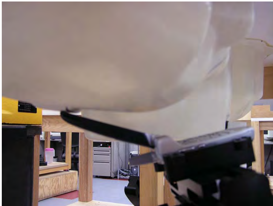
Figure 5. Phone Against the Head Phantom (15°Tilt)
