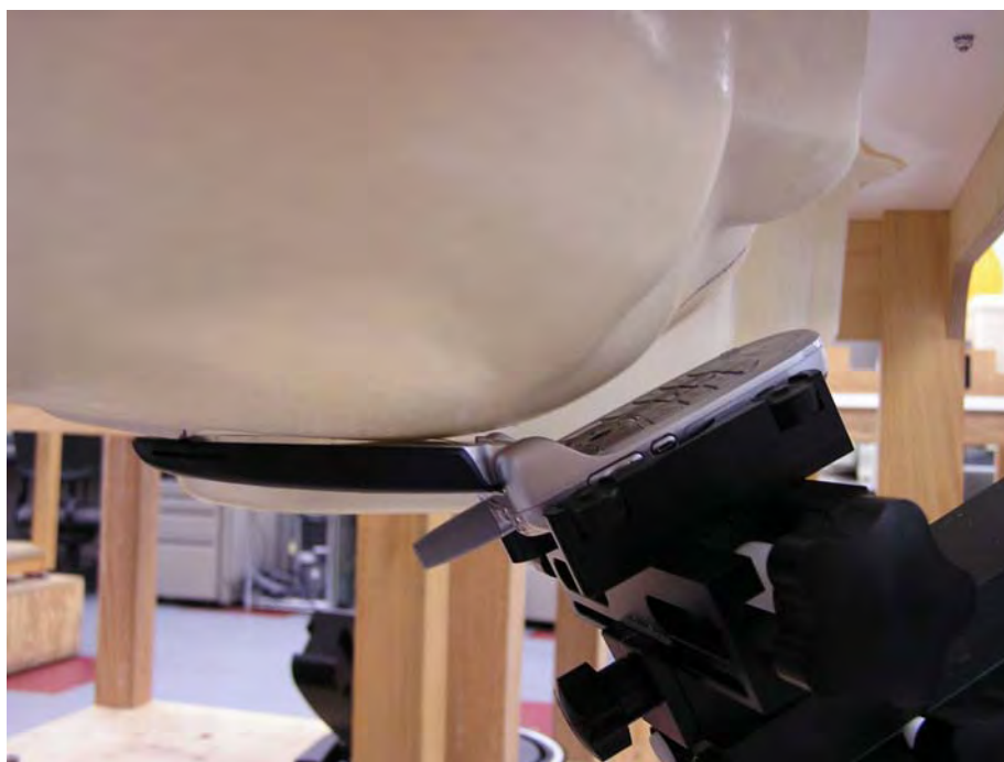
Figure 4. Phone Against the Head Phantom (Cheek Touch)
