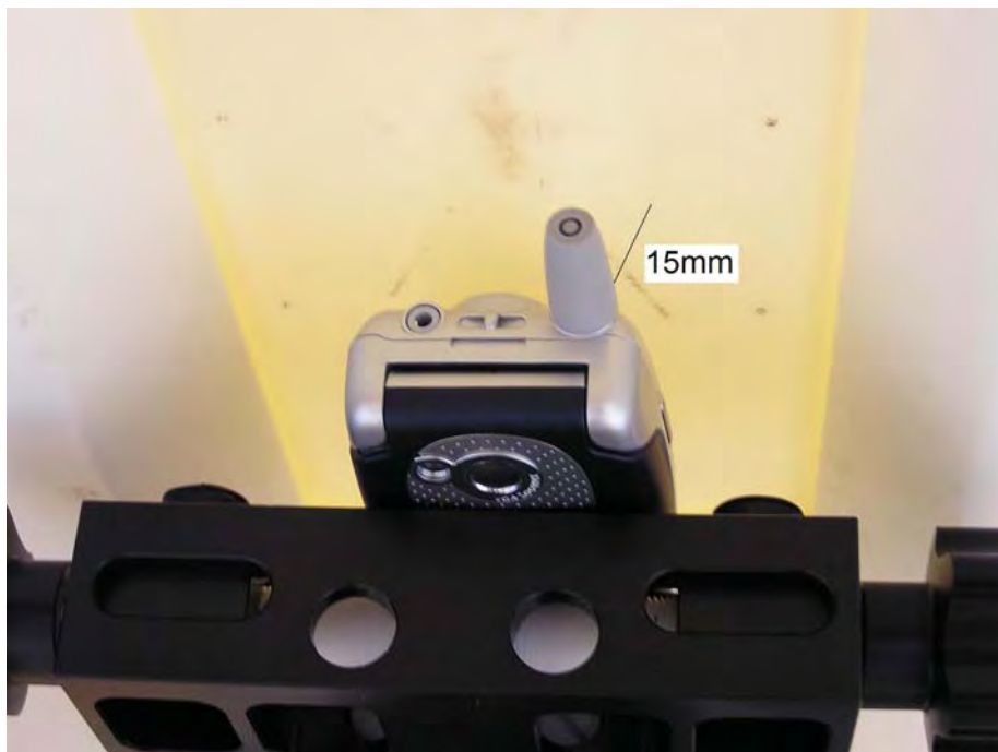
Figure 6. Phone Against the Flat Phantom
