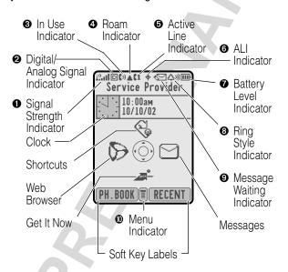
Use the 4-way navigation key ((-)) to select one of the four menu feature icons in the display. Labels at the bottom corners of the display show the current soft key functions.
