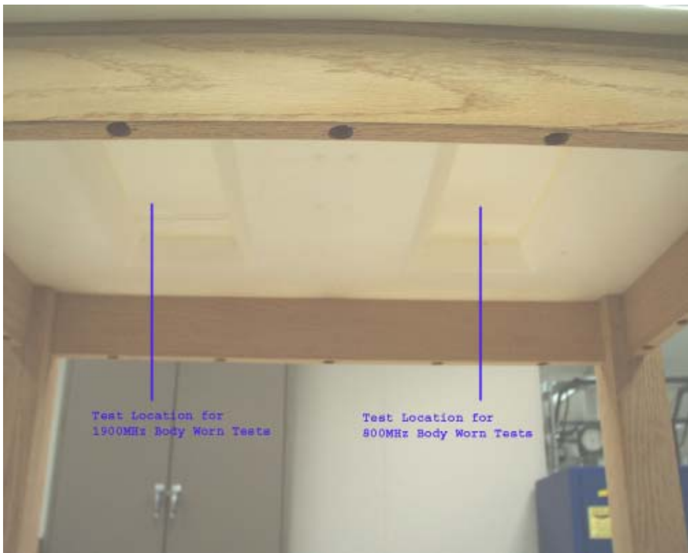
Figure 2. Underside of "Twin Tub" showing DUT placement locations.
