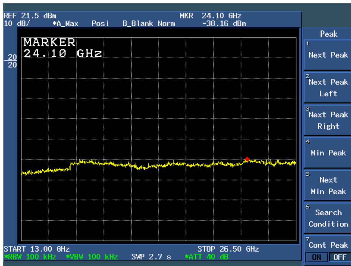
Figure 6d.7-13: Plot of spurious conducted emissions 13.0 GHz – 26.5 GHz (Hopping Enabled).
