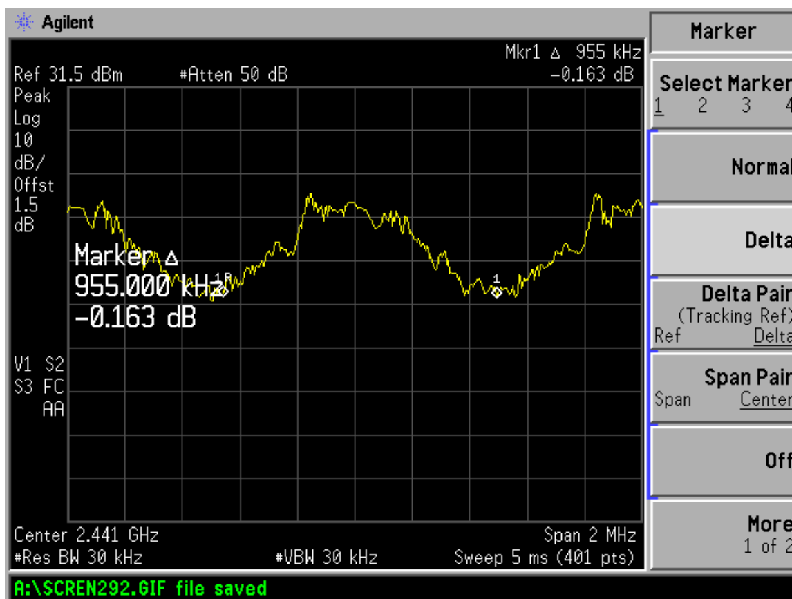
Figure 6d.2-1: Plot of 20 dB bandwidth (GFSK Modulation)
