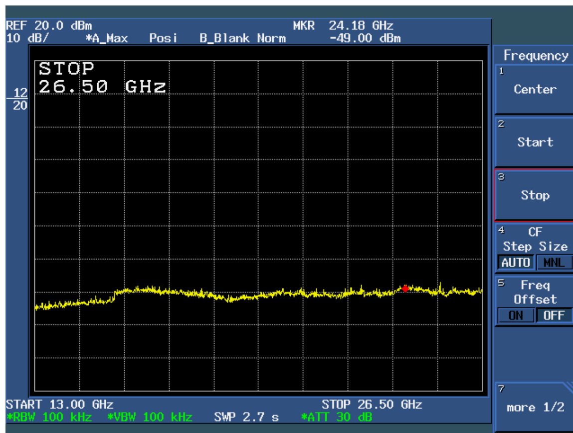
Figure 6d.7-9: Plot of spurious conducted emissions 13 GHz – 26.5 GHz (High Channel).
