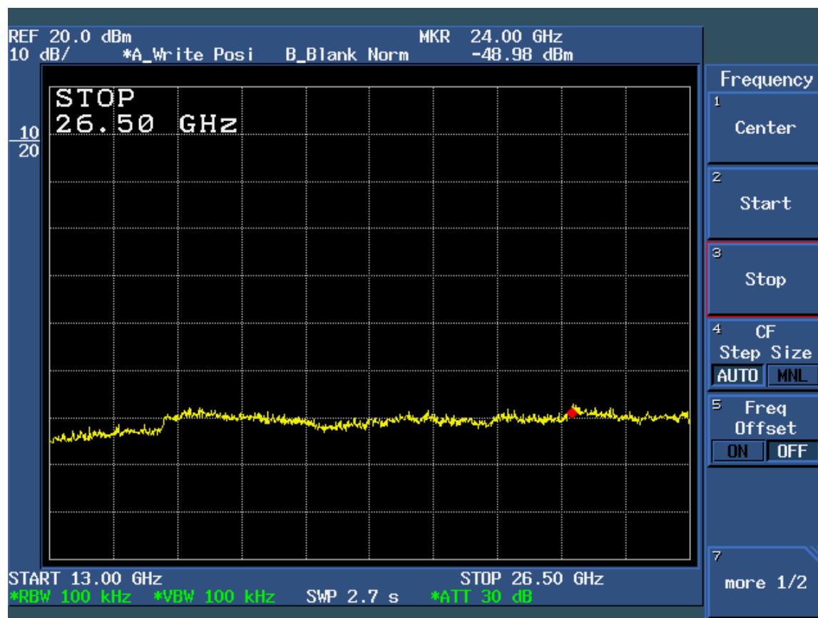
Figure 6d.7-6: Plot of spurious conducted emissions 13 GHz – 26.5 GHz (Mid Channel).
