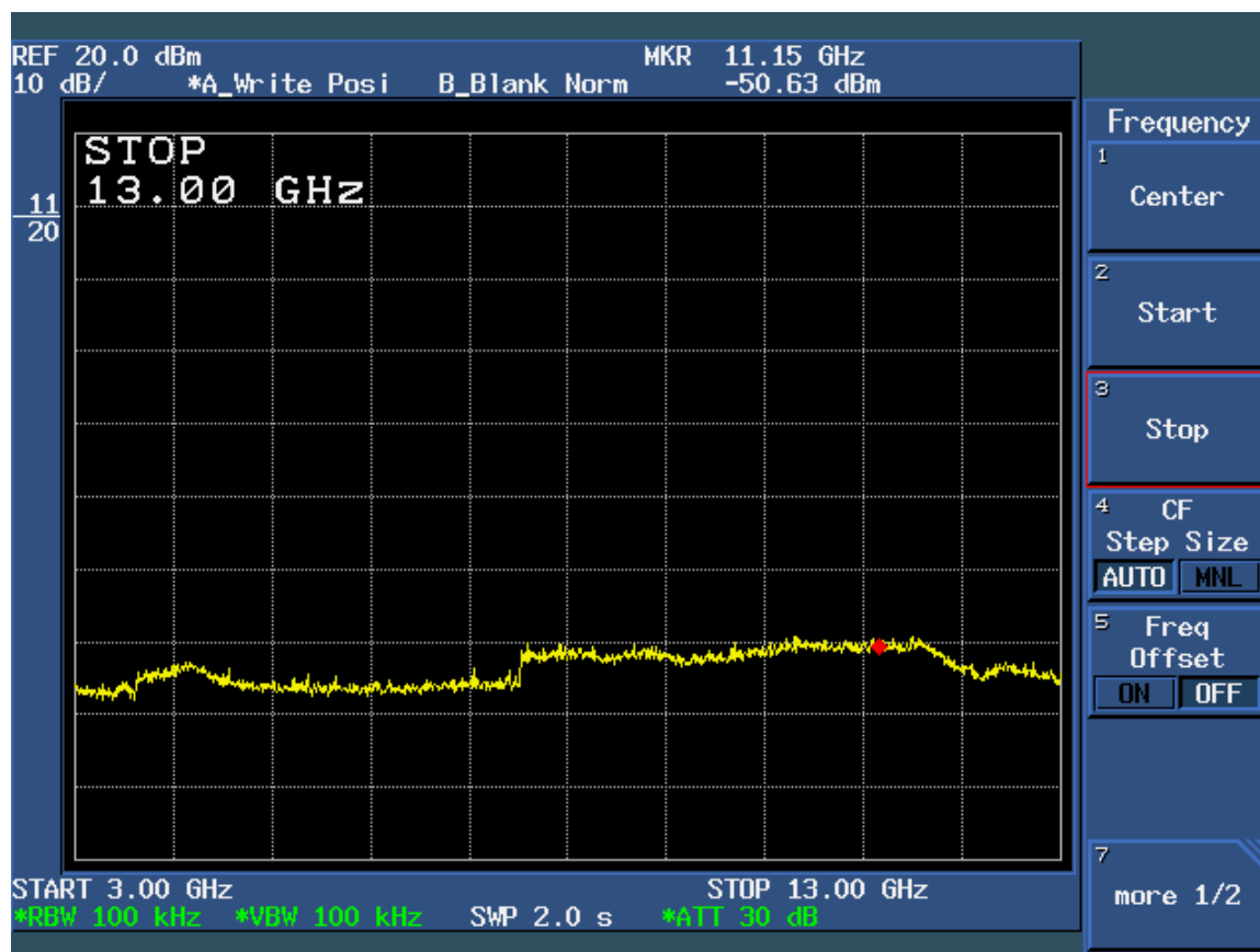
Figure 6d.7-5: Plot of spurious conducted emissions 3 GHz – 13 GHz (Mid Channel).
