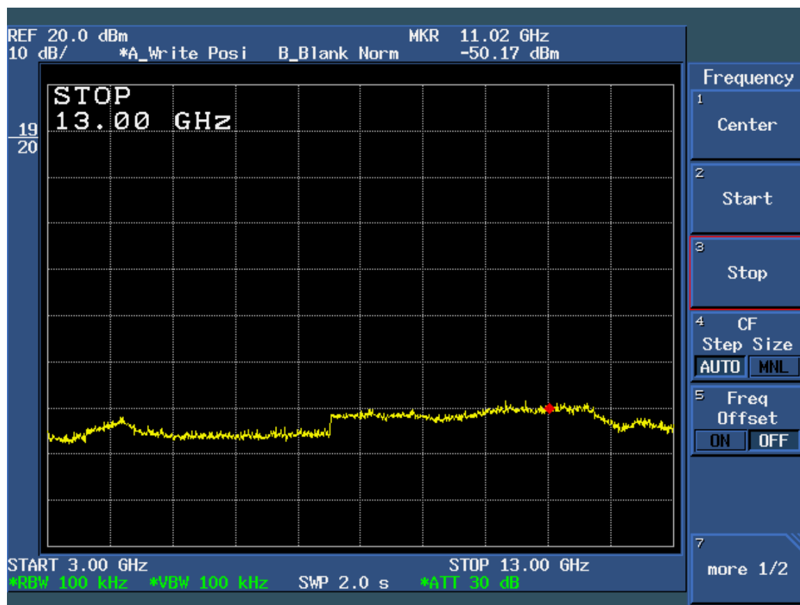
Figure 6d.7-2: Plot of spurious conducted emissions 3 GHz – 13 GHz (Low Channel).
