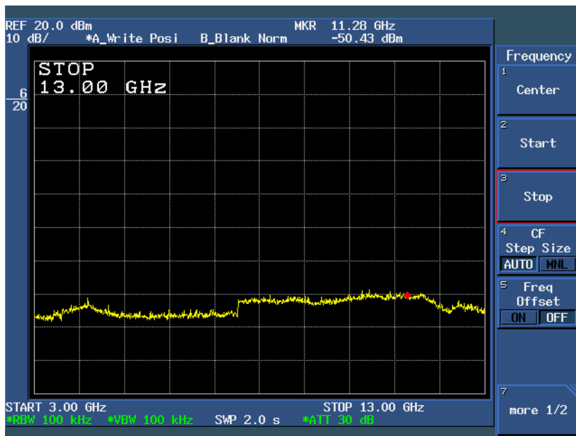
Figure 6d.7-8: Plot of spurious conducted emissions 3 GHz – 13 GHz (High Channel).
