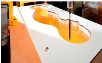
Figure 6-2 SAM Phantom with Simulating Tissue
