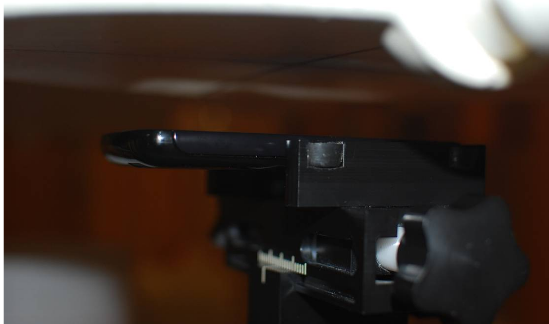
Figure 18-4 SAR Test Setup Front 2.5 cm
