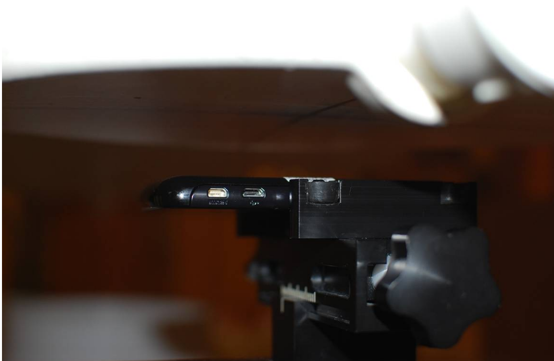
Figure 18-2 SAR Test Setup Back 2.5 cm
