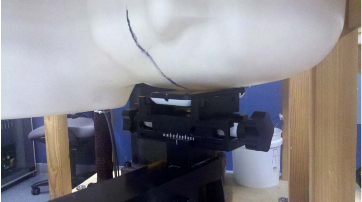
Figure 2: Cheek Position, Front of Head of Phantom
