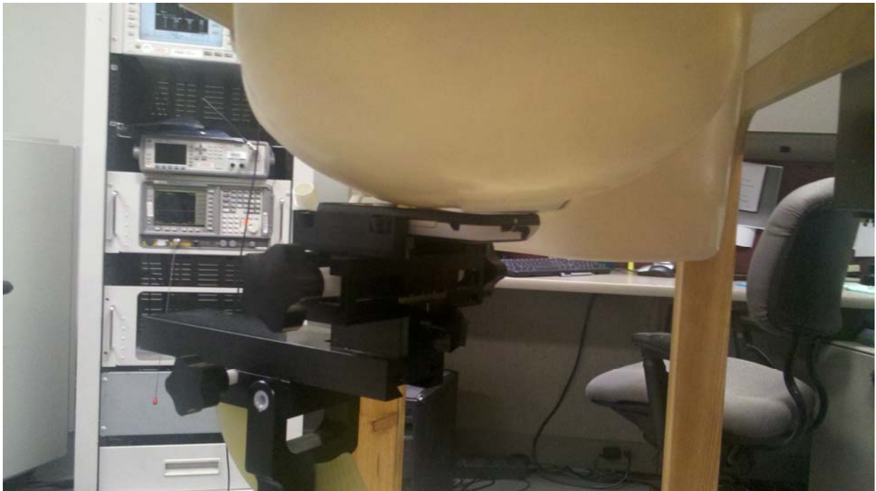
Figure 3: Cheek Position, Top of Head of Phantom
