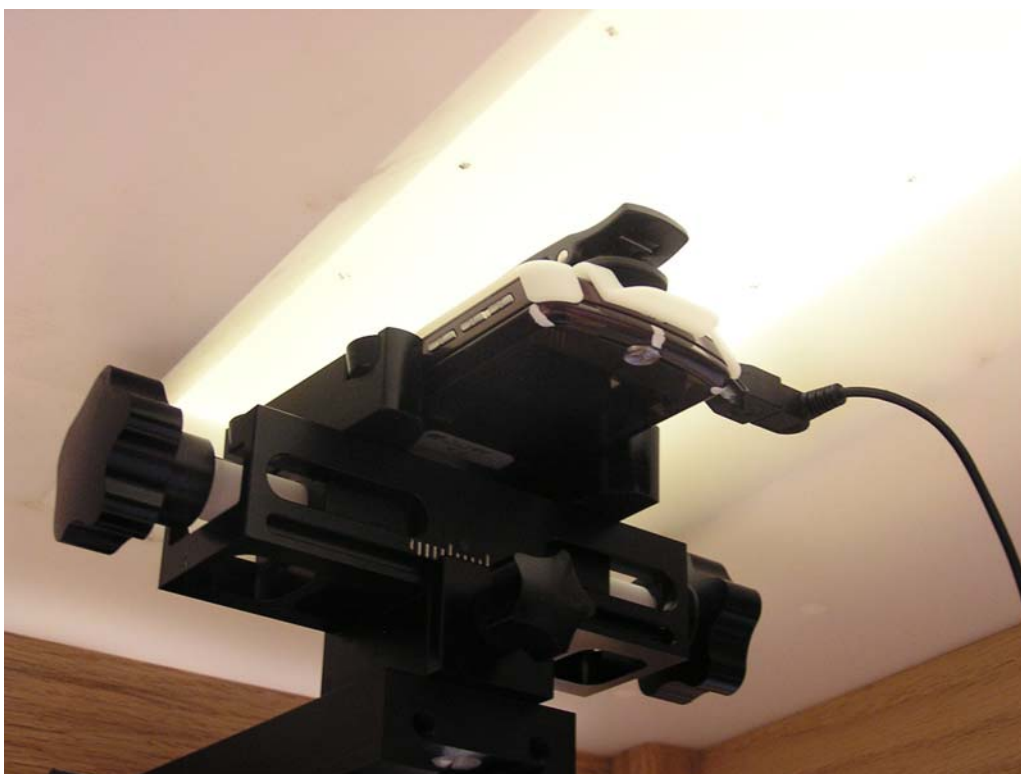
Figure 12 – Transceiver against body with Accessory
