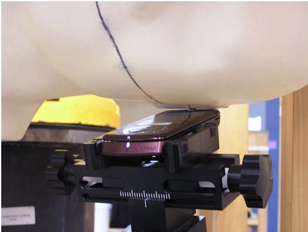
Figure 9 – Transceiver against head, 15° Tilt position, Slider Retracted
