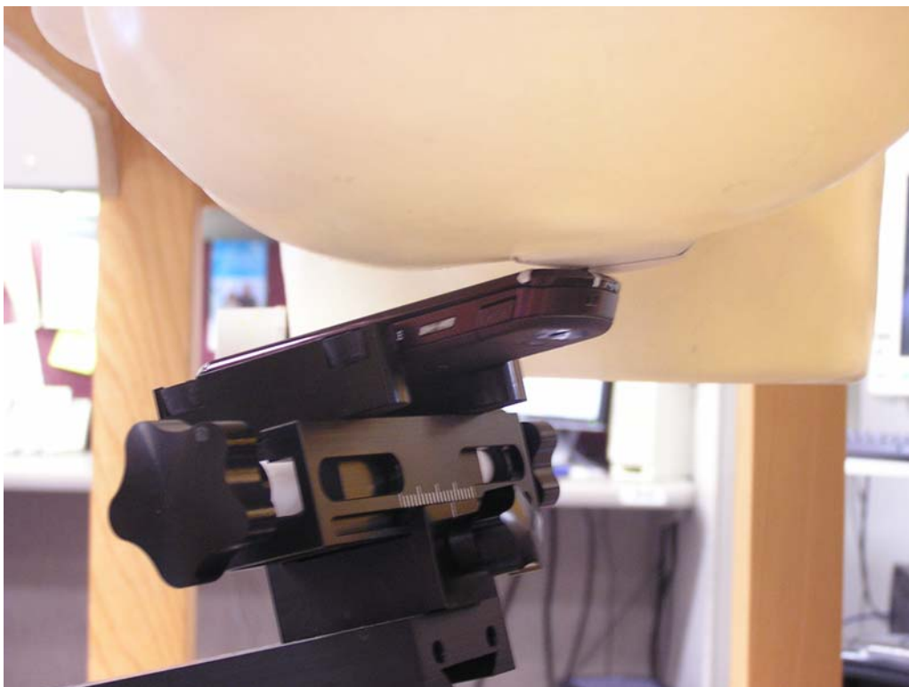
Figure 10 – Transceiver against head, 15° Tilt position, Slider Retracted
