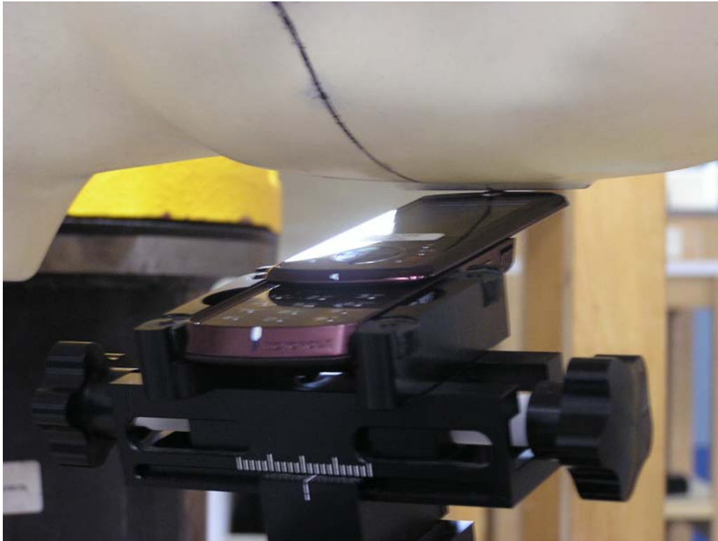
Figure 7 – Transceiver against head, 15° Tilt position, Slider Extended
