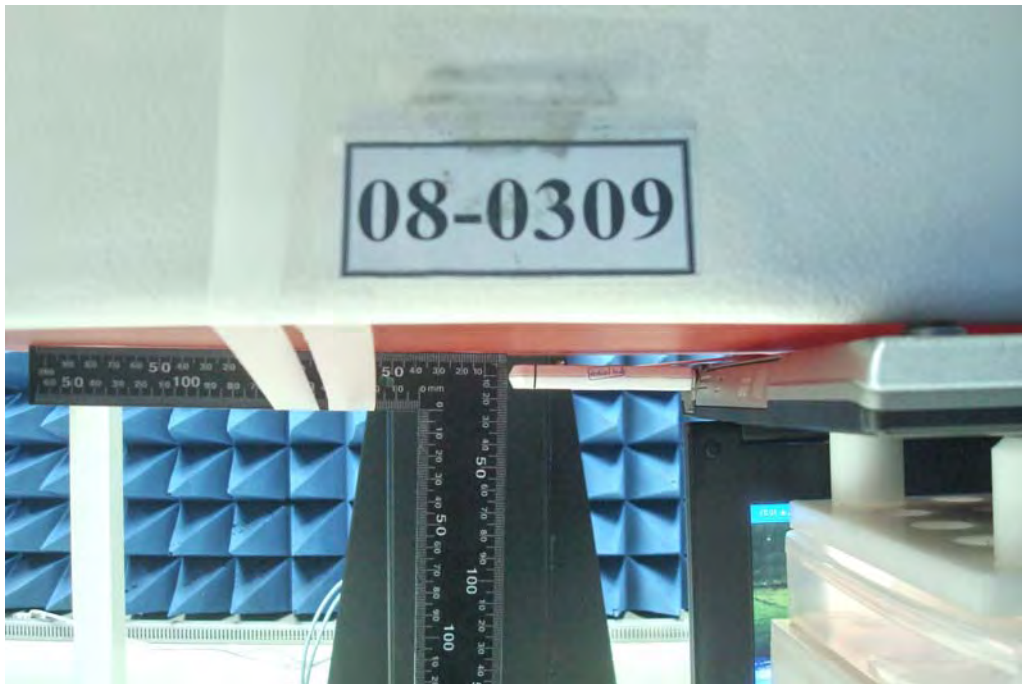
Figure 12. Body SAR Test Setup (Flat Section) _ EUT Horizontal Up_LCD Open 90°_5mm
