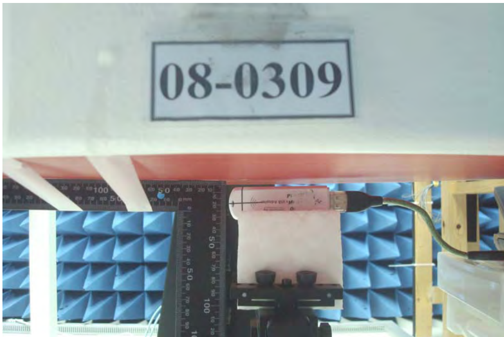
Figure 16. Body SAR Test Setup (Flat Section) _ Vertical Back with USB Cable_5mm
