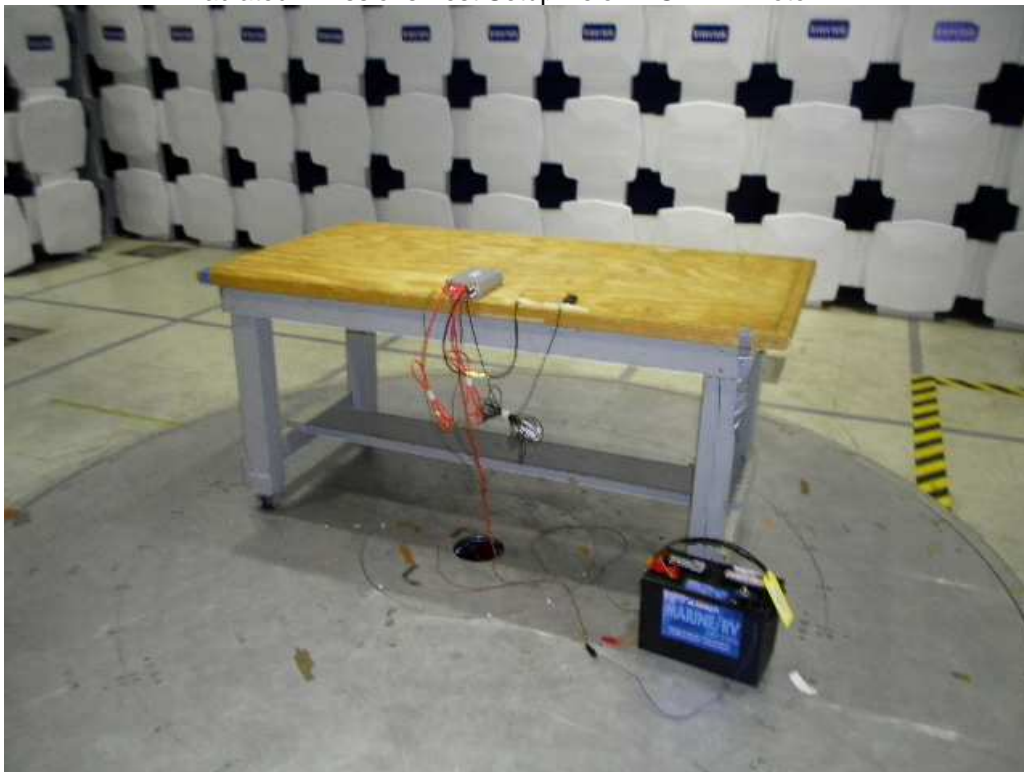
Radiated Emissions Test Setup Below 1GHz – Photo # 2
