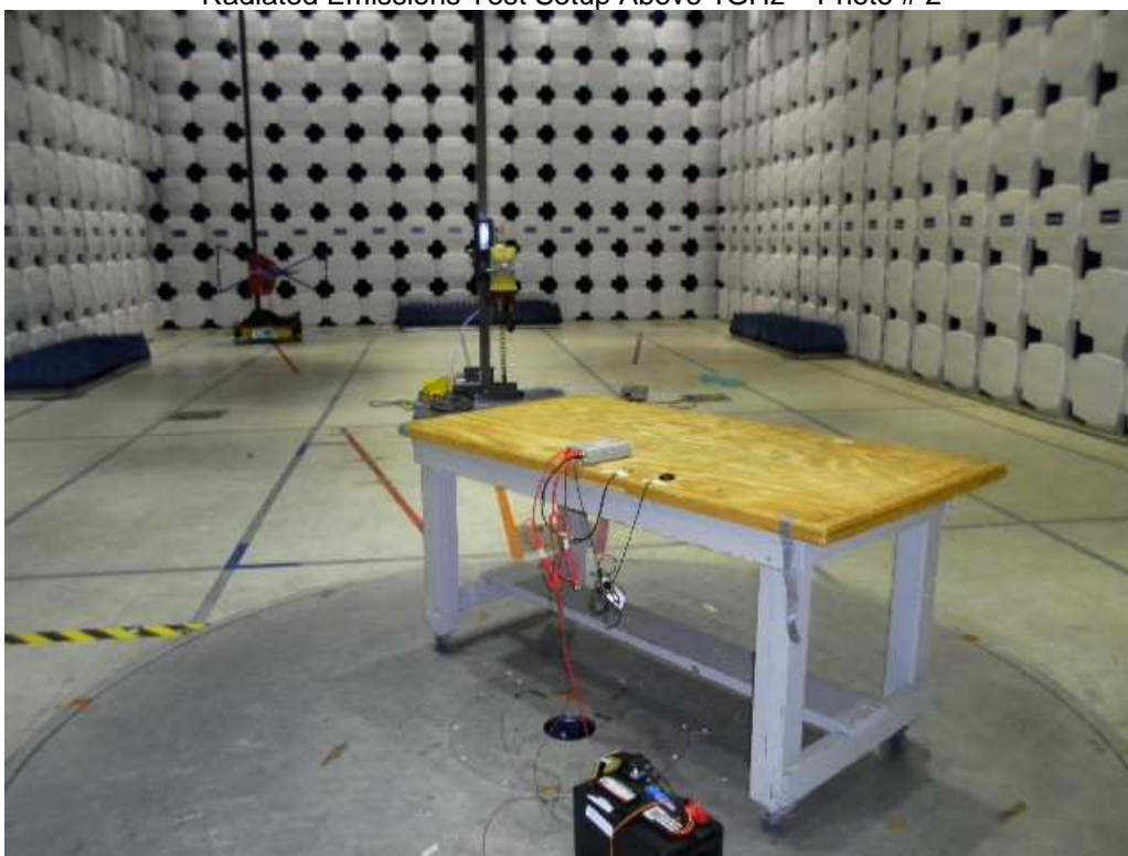
Radiated Emissions Test Setup Above 1GHz – Photo # 2
