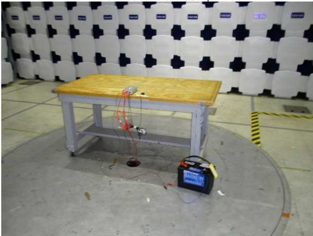
Receiver Radiated Emissions Setup Photo
