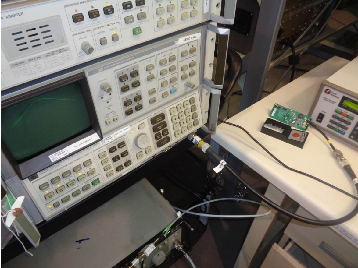
Antenna Conducted Emissions Setup Photo
