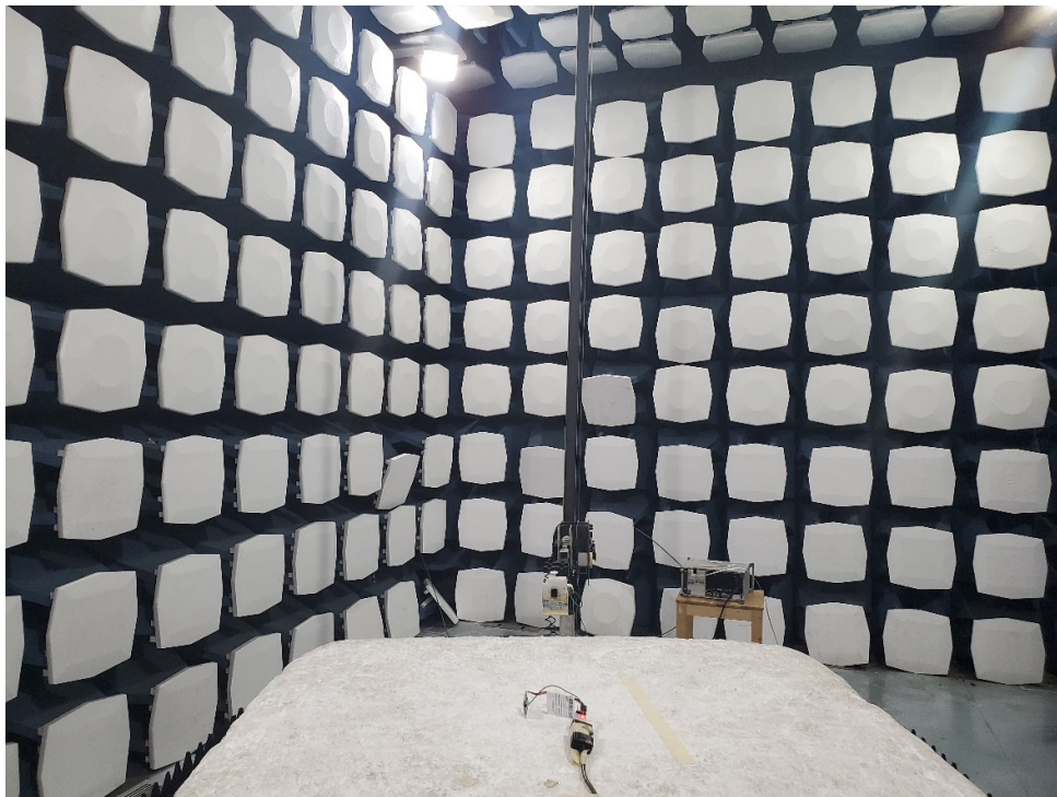
Picture 1 Radiated Emission Test Setup
