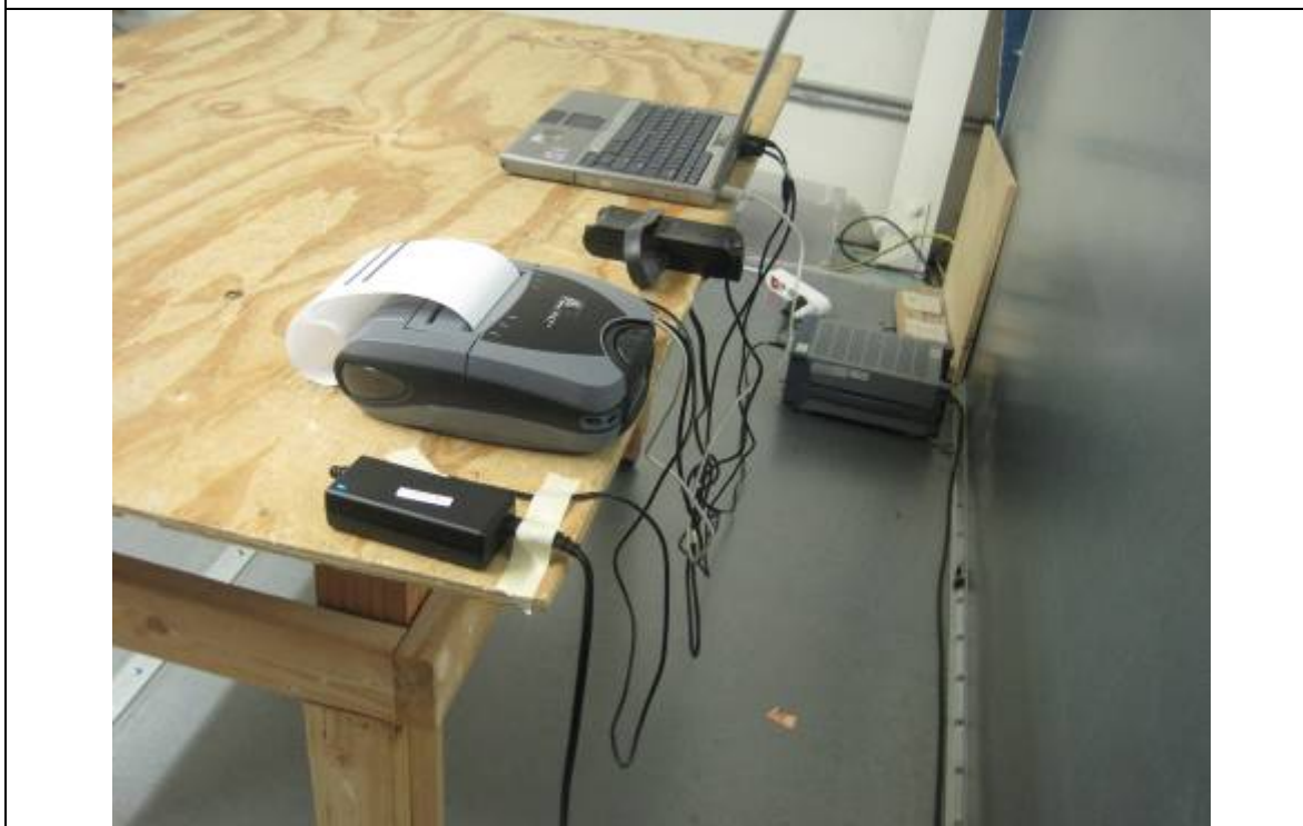
Conducted Emission Test Setup – Rear View
