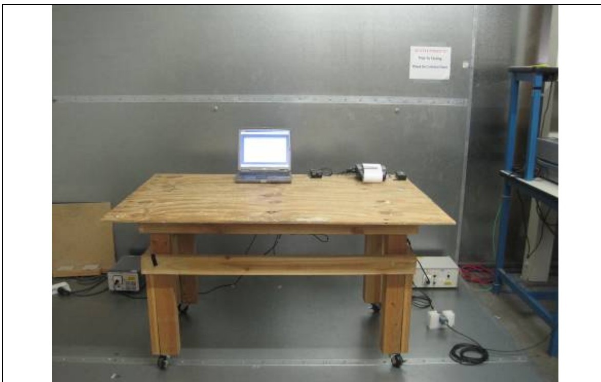
Conducted Emission Test Setup – Front View
