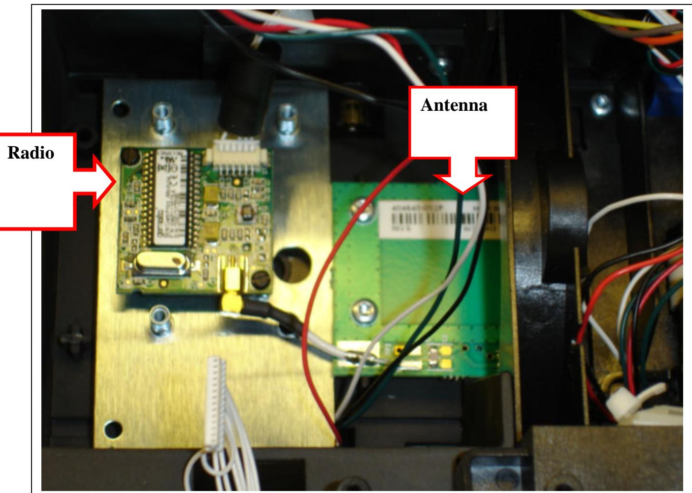
**P100i PCBA Removed from printer.
