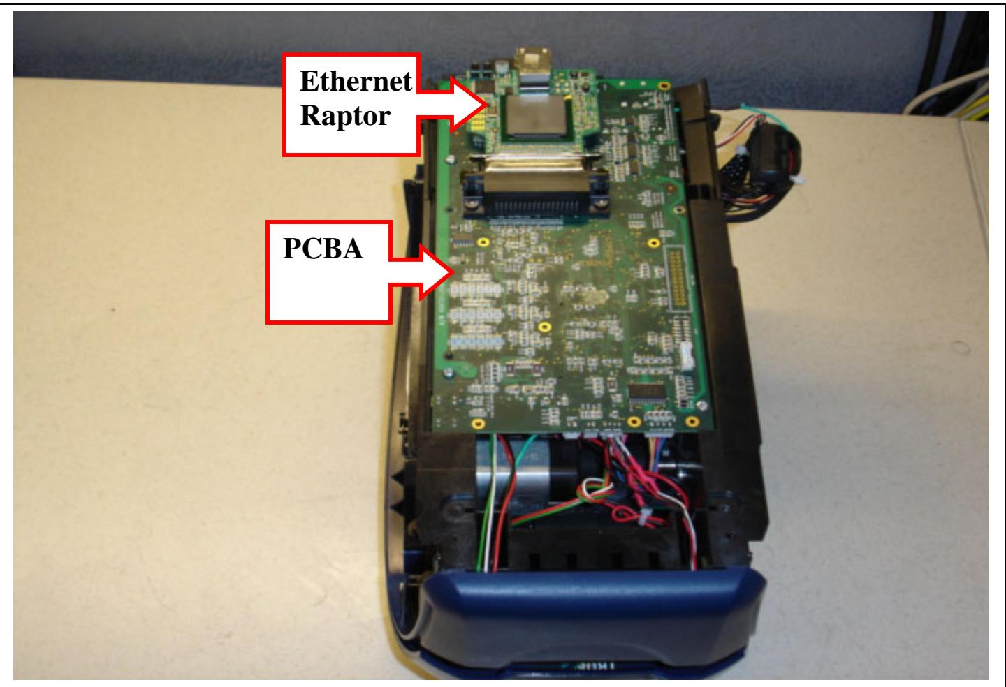
**P100i Top view of PCBA Board / Auxiliary Fan with Metal Shield.**
