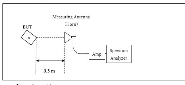
Distance Factor:  $20 \times \log (0.5 \text{ m}^* / 3.0 \text{ m}) = -15.6 \text{ dB}$
