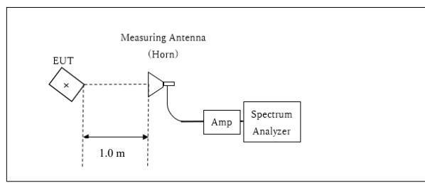
Distance Factor:  $20 \times \log (1.0 \text{ m}^* / 3.0 \text{ m}) = -9.5 \text{ dB}$
