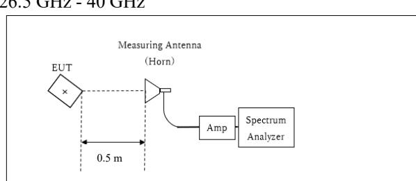
Distance Factor:  $20 \times \log (0.5 \text{ m}^* / 3.0 \text{ m}) = -15.6 \text{ dB}$
