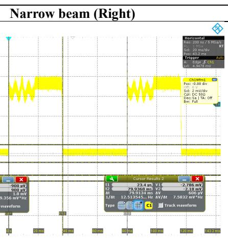
The declared duty factor and measured one were compared. The maximum duty factor of these results was applied to the average field strength measurement. (Worst case)
