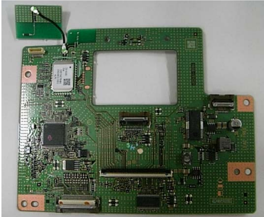
PCB including Bluetooth IC (Component Side)
