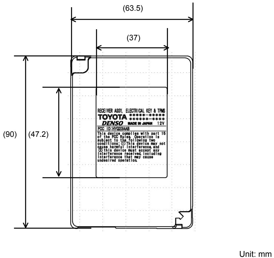
Fig. Marking location and layout of Receiver
