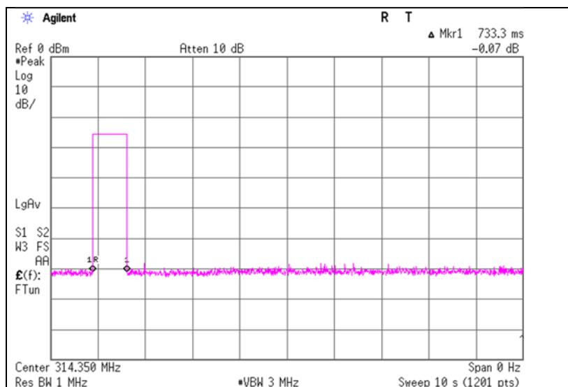
\* The EUT transmits UHF when LF signal is received from a car or a button on the EUT is pressed. In both cases, the UHF transmission is stopped within 5 seconds. So the test was performed by a button-pressed operation as the worst case. Please refer to the "Theory of Operation" for details.
