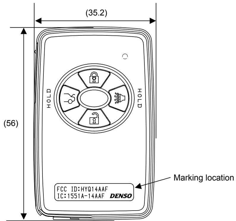
Fig. Marking location and layout of Transmitter
