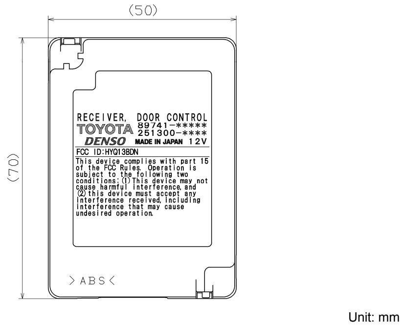
Fig. Marking location and layout of Receiver
