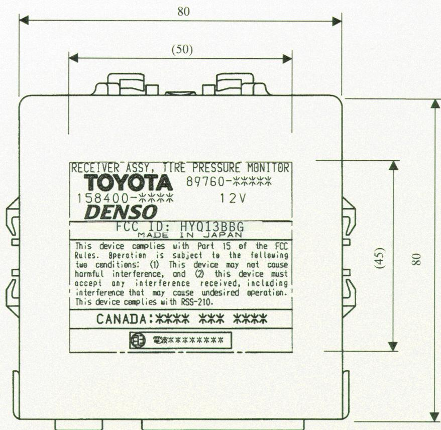
Fig7-1. Marking location and layout of receiver
