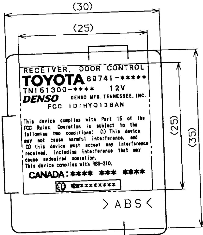
Fig. Marking location and layout of receiver
