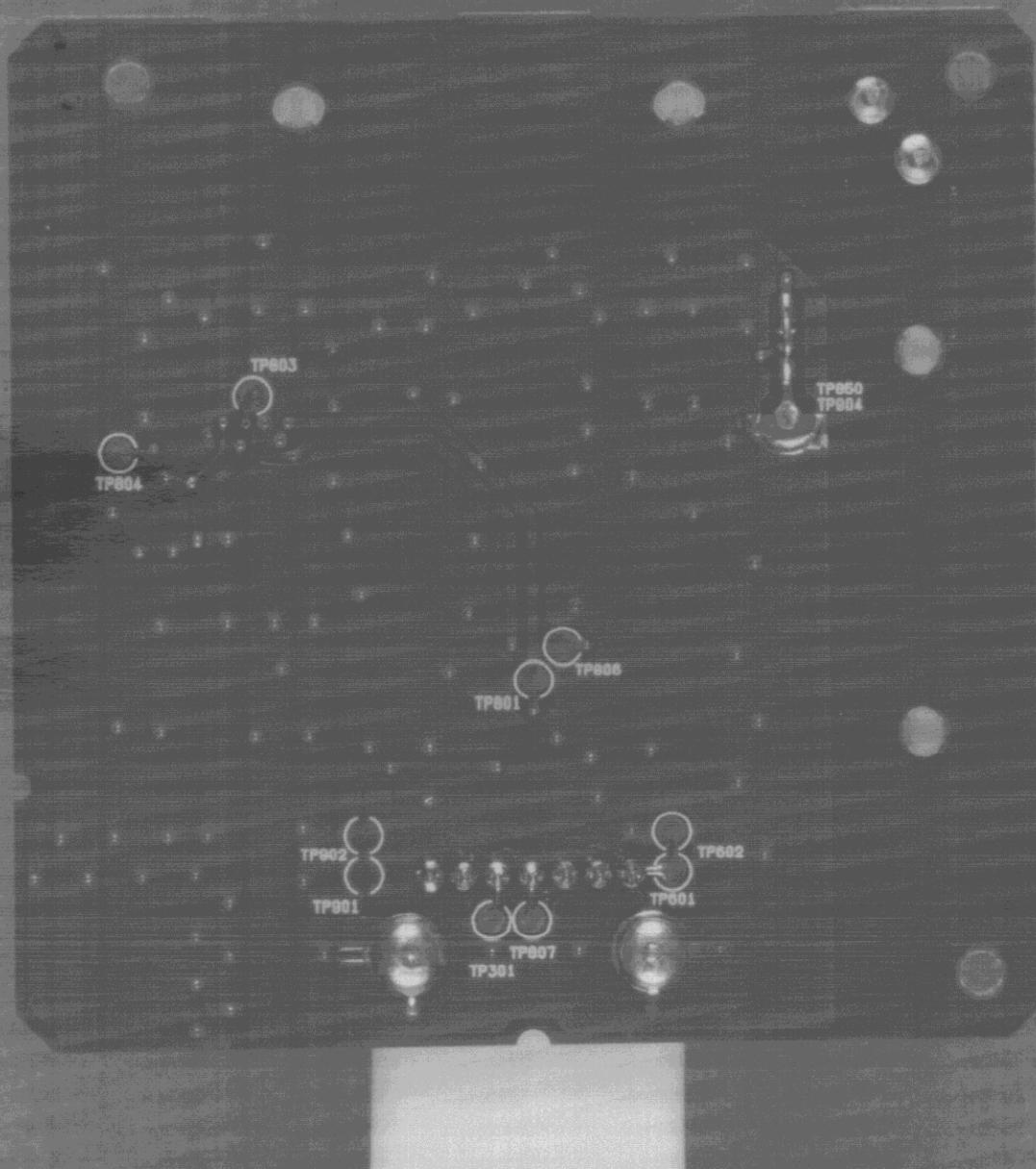
PCB Solder side view of Receiver
