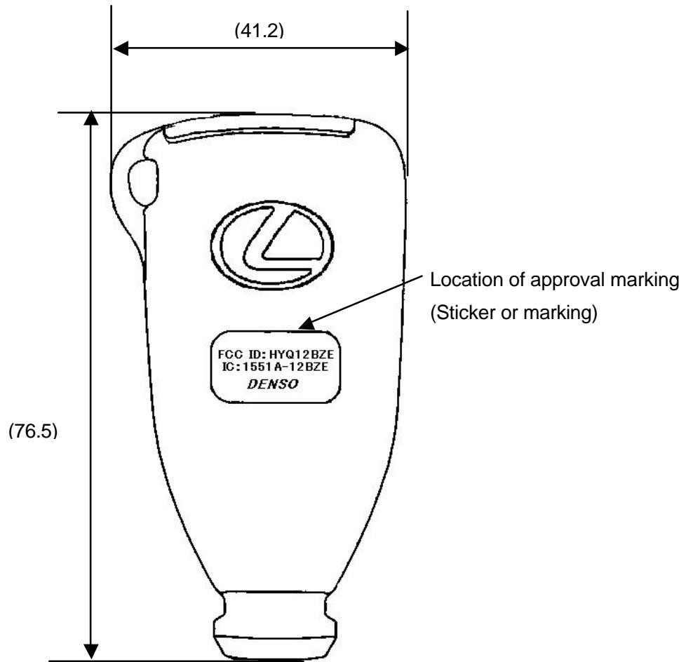
Fig. Marking location and layout of Transmitter
