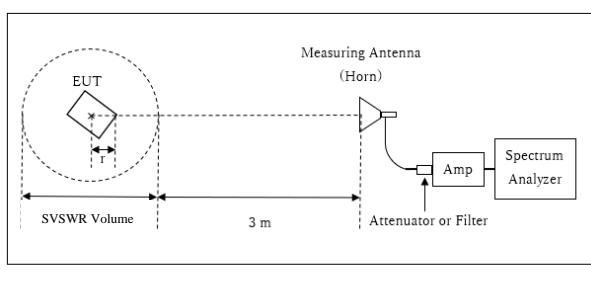
Distance Factor:  $20 \times \log (4.00 \text{ m}^*/3.0 \text{ m}) = 2.50 \text{ dB}$
