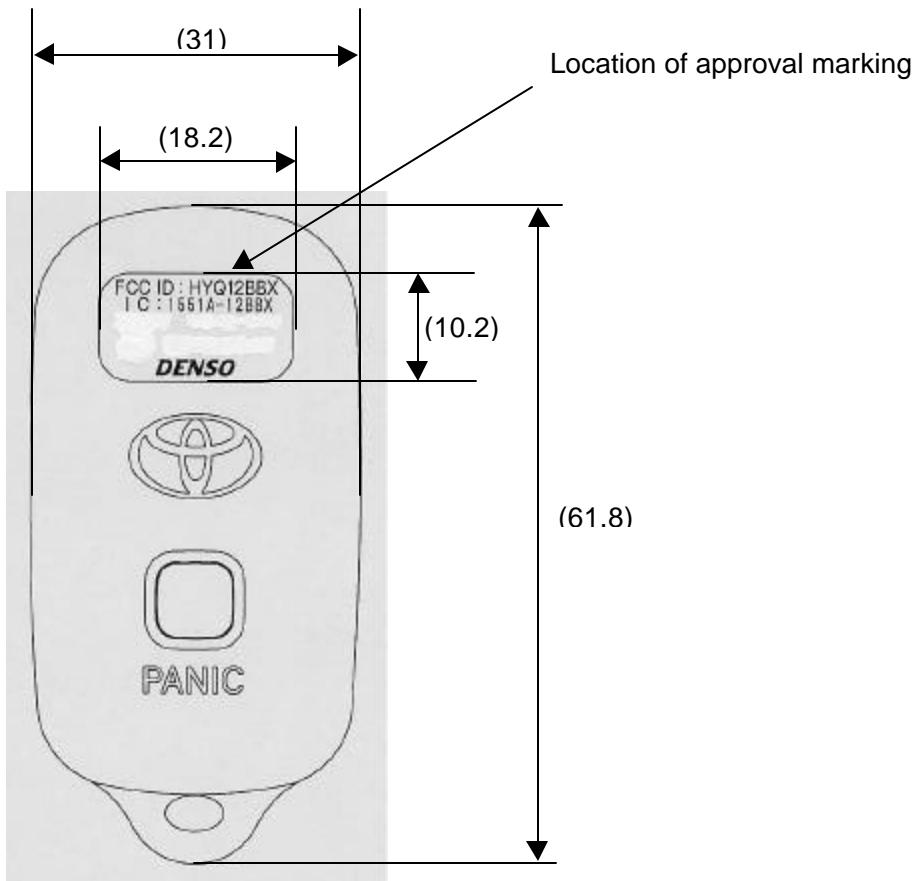
Fig. Marking location and layout of Transmitter
