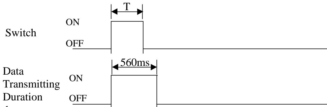
The transmitter sends the data till 560ms from the switch ON.
