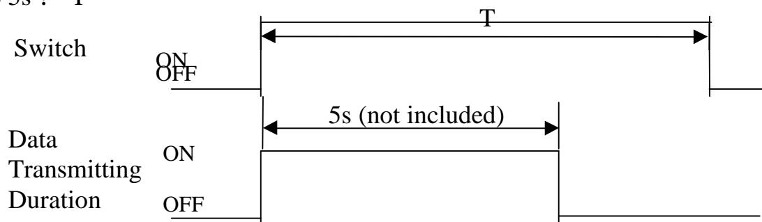
When the switch is pressed for more than 5s, the transmitter stops sending the data in 5s (not included) from switch ON. (Auto-power off function)
