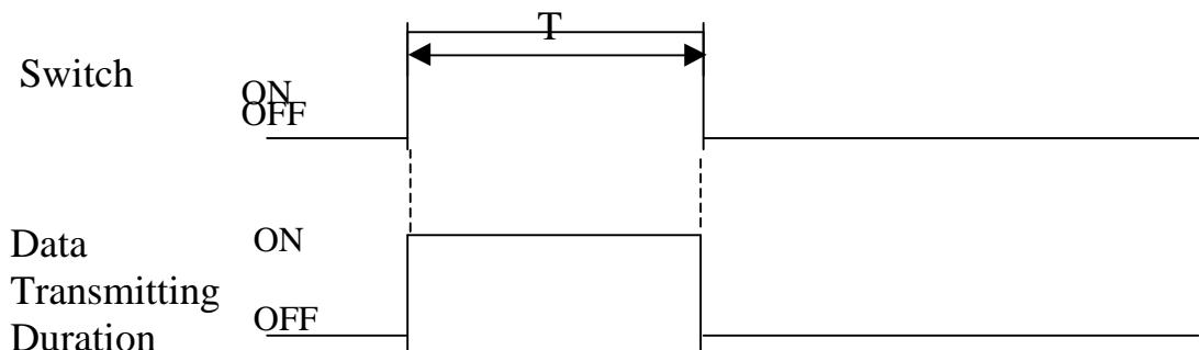
The transmitter sends the data while the switch is pressed.
