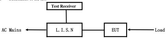
**EUT: Equipment Under Test**
