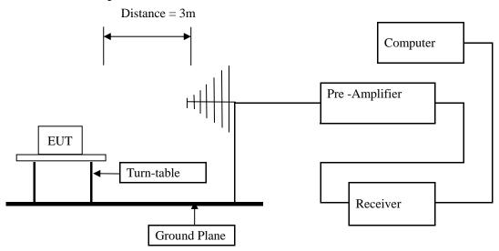
For the actual test configuration , please refer to the related items – Photos of Testing The deactivation test was performed in the 3 meters chamber B test site, using the setup accordance with the ANSI C63.4 - 2009. The specification used was the FCC 15.231(e) limits.
